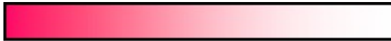
Fig. 1. Heat Flow in a Rod. The regulation of the temperature profile of a rod is the simplest example of a control system modelled by a partial differential equation. The control action can be effected by varying the heat flow at one end (Neumann boundary conditions) or by keeping the temperature at one end fixed (Dirichlet boundary conditions). The temperature is measured at some point along the rod. The choice of these boundary conditions and the measurement position affect the location of the poles and zeros of the system significantly.
