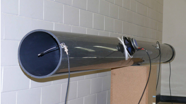
Fig. 3. Acoustic noise in a duct. A noise signal is produced by a loudspeaker placed at one end of the duct. In this photo a loudspeaker is mounted midway down the duct where it is used to control the noise signal. The pressure at the open end is measured by means of a microphone as shown in the photo. How the behavior of the acoustic waves at the open end is modeled affects the location of the poles significantly. (Photo by courtesy of Prof. S. Lipshitz, University of Waterloo)
