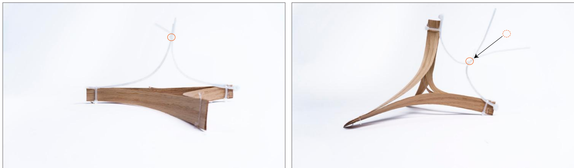
Module 01: Testing torsion and bending properties of a four sided module.
