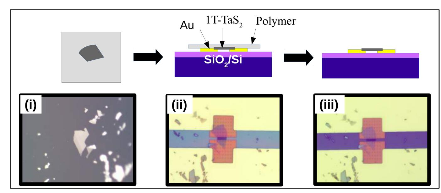
• A polymer-based exfoliation and transfer technique is used to fabricate the samples.
