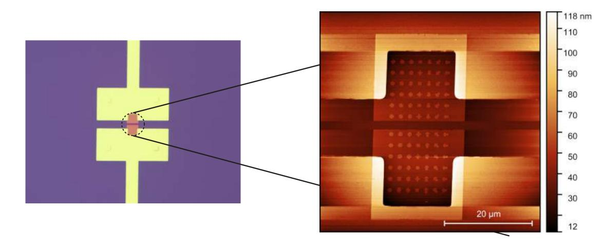
• The electrodes were fabricated using electron beam lithography and imaged using atomic force microscopy.
