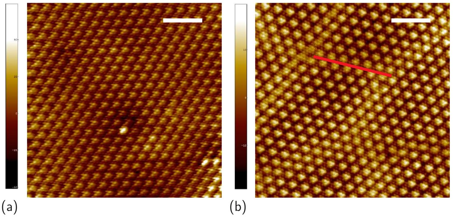
STM images of bulk 1T- $TaS_2$  in the C phase at 77 K (a) and the NC phase at 200 K (b) (scale bar = 4 nm). The arrangement of charge density wave "stars" in the C phase is highly uniform, while in the NC phase domains of C phase are separated by a period of dis-commensuration (e.g. along the red line in (b)).
