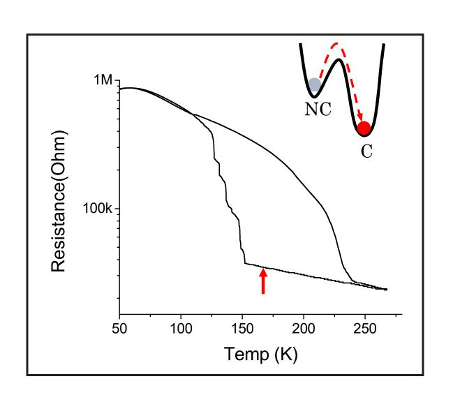
•In thin samples it is possible to drive the material from the NC phase towards the C phase by passing current through the sample.
