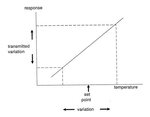
The first strategy is to reduce the variation in the noise factor. If the temperature range was reduced by half, as in the next figure, the transmitted variation is also reduced. If the size of an incoming part to a machining operation affects the outgoing critical dimension, then process variation can be lessened by reducing variation in the incoming size. This strategy may be difficult and expensive to implement. It corresponds to the maxim "move quality improvement upstream".
