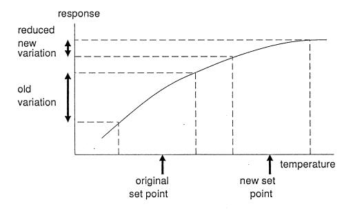
There may be several problems with this approach. High costs may be incurred by moving the specification. It may be impossible to find a "flat" spot in the response graph. Changing the set point of the temperature may also move the process mean away from the target, and hence another control parameter would have to be shifted to recentre the process. Finally, changing the temperature may adversely affect some other quality characteristic so that one problem is merely replaced by another.
