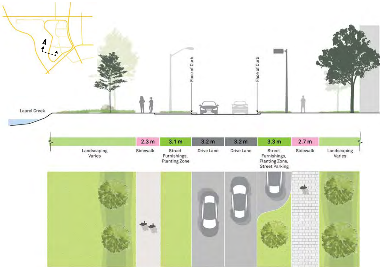
Figure 55. Section A. Existing condition of Ring Road (western edge).
