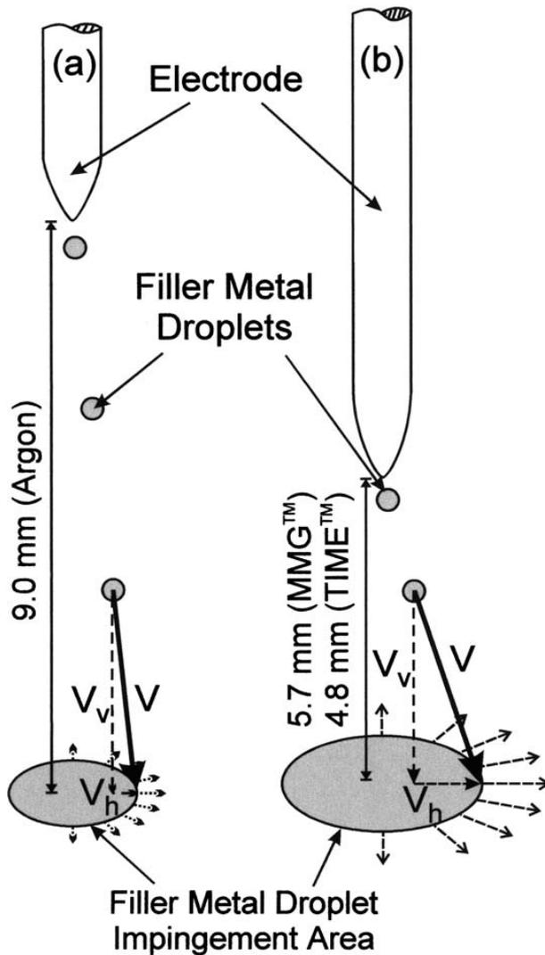
17 Difference in the overall velocity  $V$ , as well as the difference in horizontal and vertical velocity components  $V_h$  and  $V_v$ , of the filler metal droplets when using a argon and b MMG or TIME shielding gases
