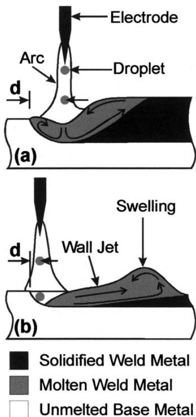
a Low welding speed; b High welding speed
