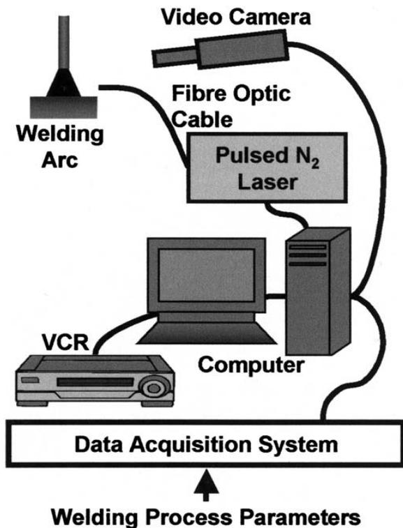
3 Various components of the LaserStrobe video imaging system
