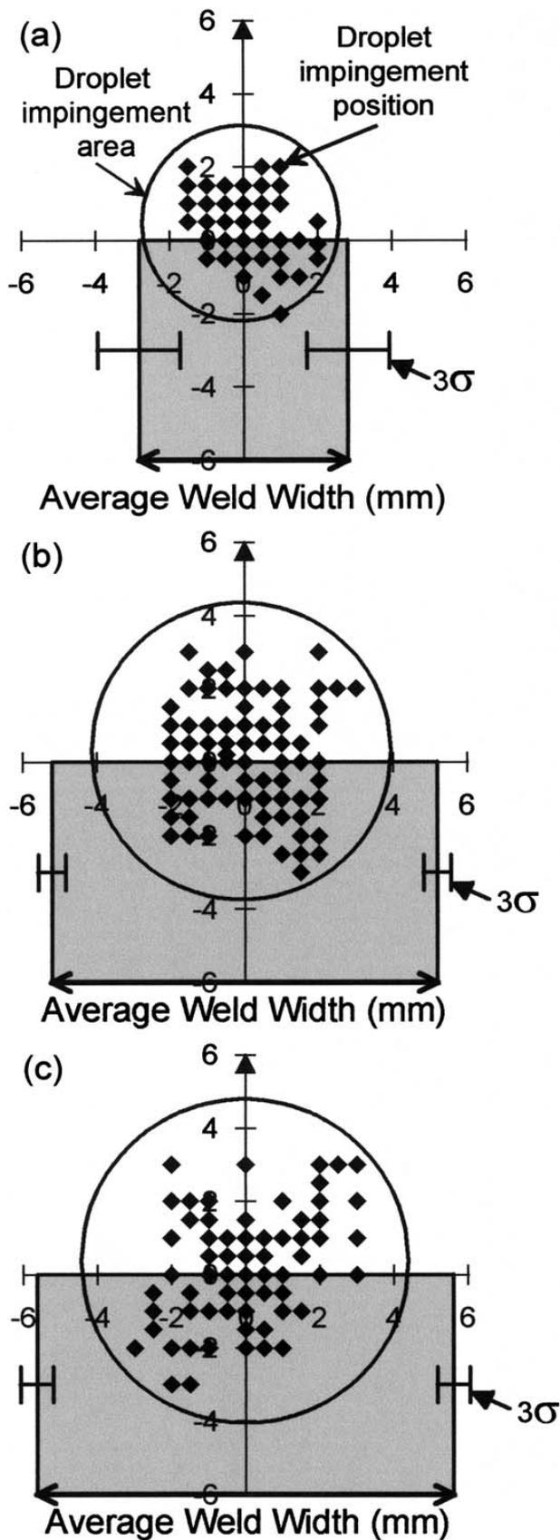
15 The filler metal droplet impingement positions and areas and the average width of welds produced using 7.5 kW welding power and 11 mm s<sup>-1</sup> welding speed in the flat position when using a argon, b MMG and c TIME shielding gases
