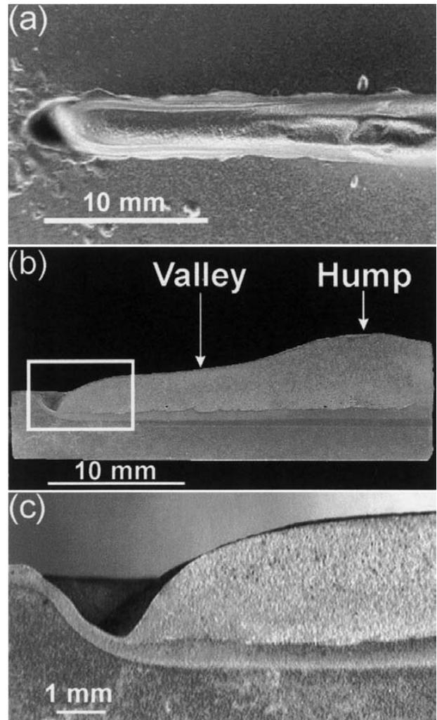
a Top view; b Longitudinal section; c Close-up view of the gouged weld pool
