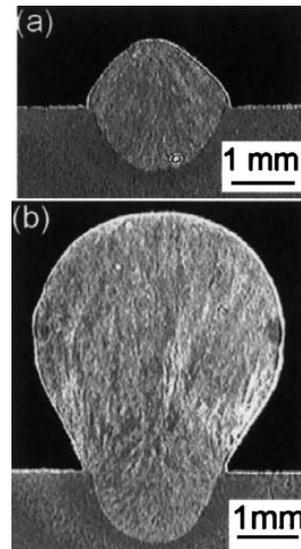
2 Transverse sections of the GMA weld shown in Fig. 1 at a valley and b a hump
