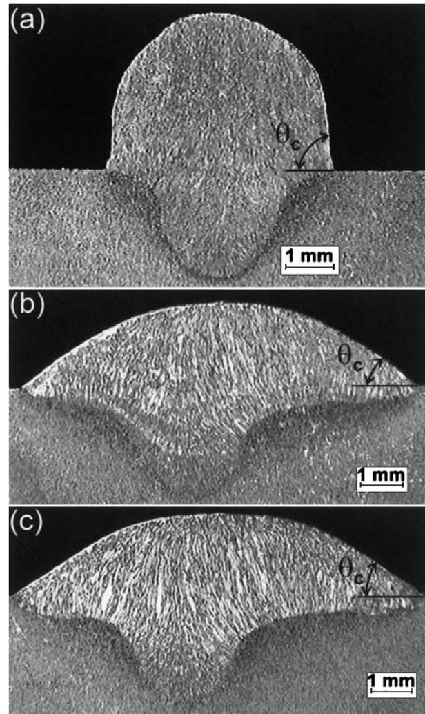
**14 Transverse sections of bead on plate GMA welds produced using 7.5 kW welding power and  $11 \text{ mm s}^{-1}$  welding speed in the flat position with a argon, b MMG and c TIME shielding gases.  $\theta_c$  is the contact angle**
