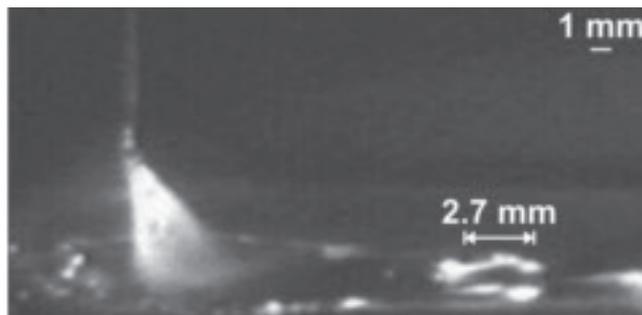
Fig. 20 — LaserStrobe™ video image that shows the length of the depression formed.
