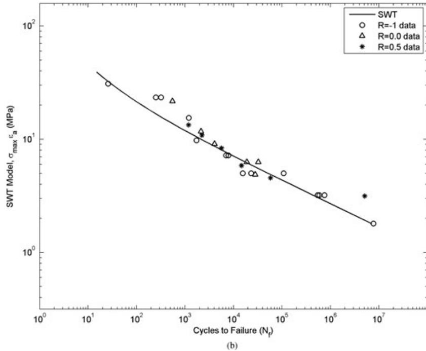
**Fig. 6** (a) Comparison of the Morrow model for various strain ratios with experimental fatigue data of 1045 HRC55. (b) Comparison of the SWT model for various strain ratios with experimental fatigue data of 1045 HRC55. (c) Comparison of the SWT model for various strain ratios with experimental fatigue data of 1045 HRC55.
