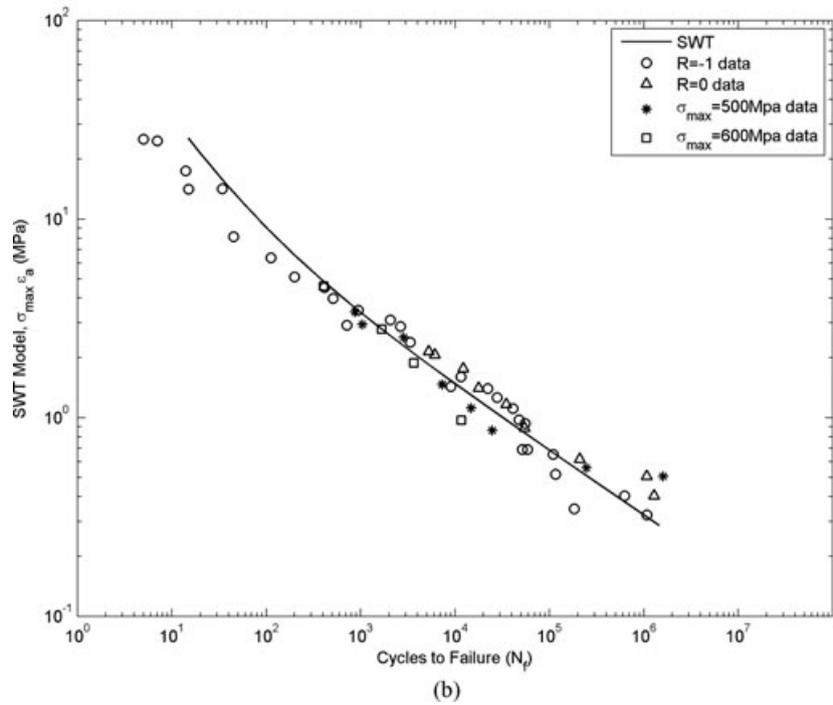
**Fig. 4** (a) Comparison of the Morrow model with experimental mean stress fatigue data of 7075-T651. (b) Comparison of the SWT model with experimental mean stress fatigue data of 7075-T651. (c) Comparison of the proposed model with experimental mean stress fatigue data of 7075-T651.
