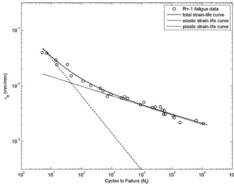
**Fig. 2** Experimental fatigue data and the fitted strain-life curve for the 7075-T651 aluminium alloy.
