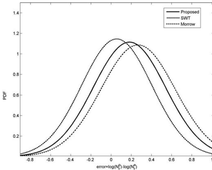
Fig. 10 Probability density function of prediction errors 1045 HRC 55 steel.
