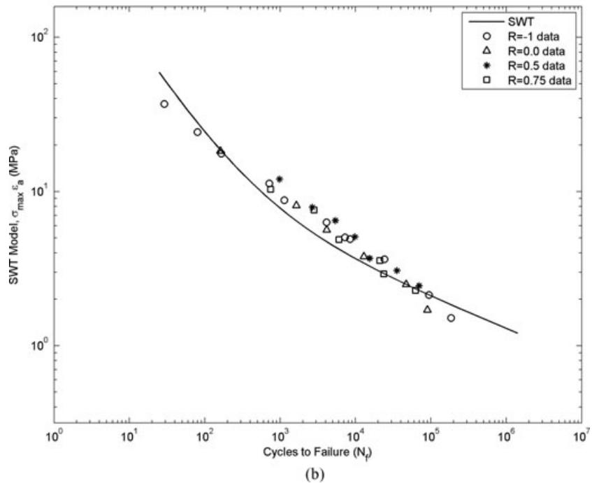
**Fig. 5** (a) Comparison of the Morrow model for various strain ratios with experimental fatigue data of ASTM A723. (b) Comparison of the SWT model for various strain ratios with experimental fatigue data of ASTM A723. (c) Comparison of the proposed model for various strain ratios with experimental fatigue data of ASTM A723.
