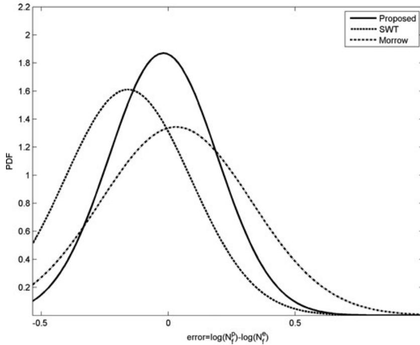
Fig. 9 Probability density function of prediction errors for ASTM A723 steel.
