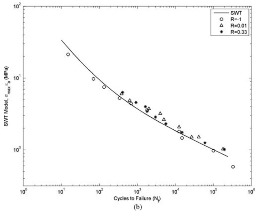
**Fig. 3** (a) Comparison of the Morrow model for various strain ratios with experimental fatigue data of Incoloy 901. (b) Comparison of the SWT model for various strain ratios with experimental fatigue data of Incoloy 901. (c) Comparison of the proposed model for various strain ratios with experimental fatigue data of Incoloy 901.
