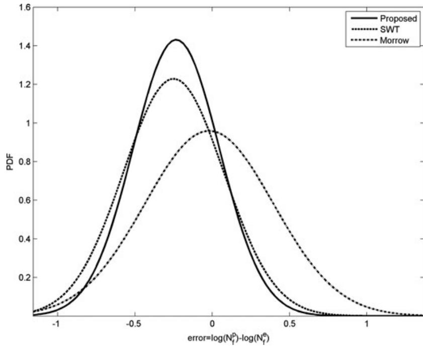
Fig. 8 Probability density function of prediction errors for 7075-T651 aluminium.
