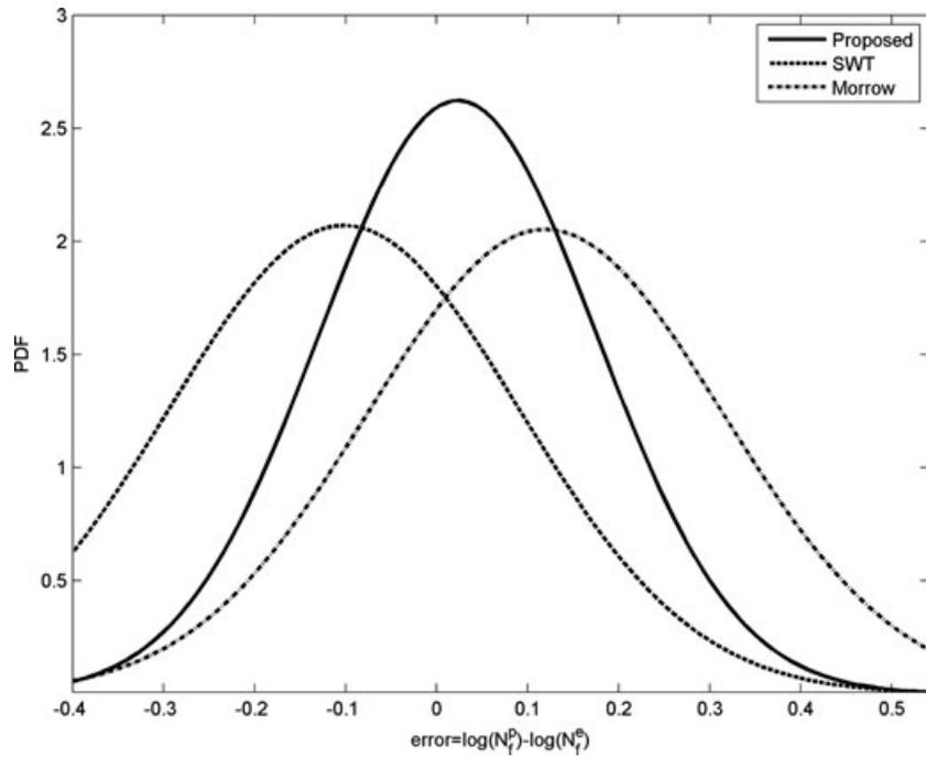
Fig. 7 Probability density function of prediction errors for the Incoloy 901 superalloy.
