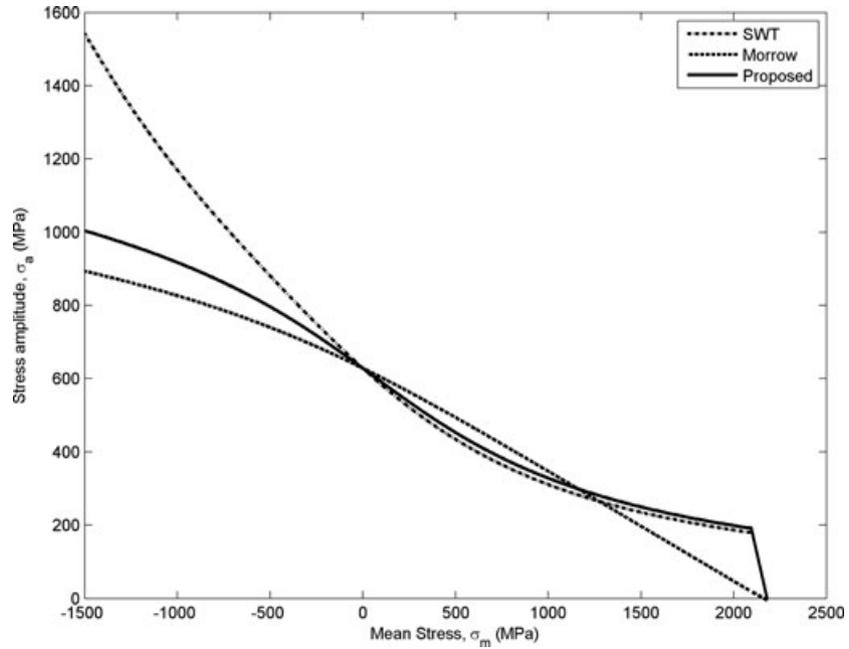
Fig. 1 Stress amplitude versus mean stress diagram for constant fatigue life of  $N_f = 1000\ 000$ – SAE 8620 alloy steel.
