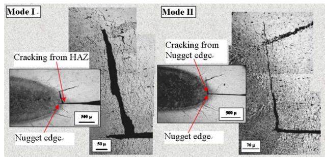
Fig. 4 Two modes of fatigue crack initiation in spot welded joints
