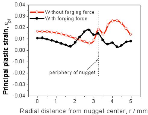
**Fig. 9 Distribution of the first principal residual plastic strain  $\epsilon_{p1}$  in the radial direction**
