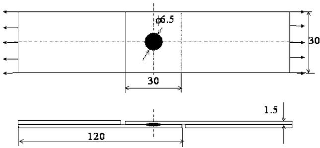
**Fig. 1** Shape and dimensions of the overlapped spot welded joints (unit: mm)
