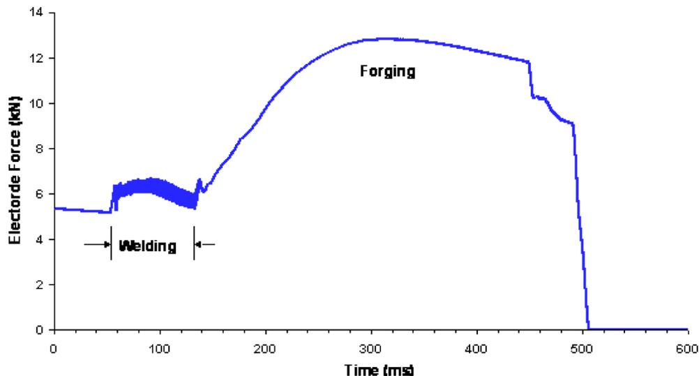
**Fig. 2** Variations of electrode force and electric current during RSW process
