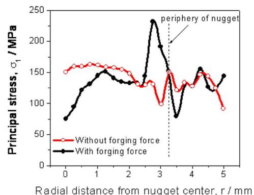
Fig. 8 Distribution of the first principal residual stress  $\sigma_1$  in the radial direction
