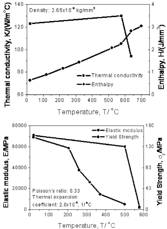
Fig. 7 Materials properties used in finite element analysis: (a) material properties for thermal analysis and (b) material properties for thermal mechanical analysis
