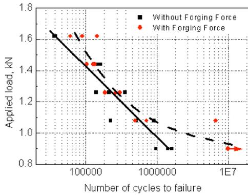
Fig. 3 Fatigue test results for the two types of joints
