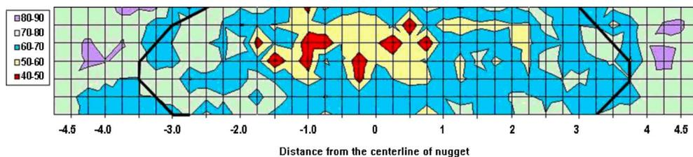
Fig. 5 The microhardness pattern of spot welds; the black lines show the boundary between the weld and surrounding area
