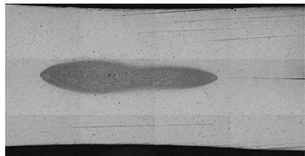
5 Shape of nugget after RSW of AA5182 with 20 kA for 1 current cycle
