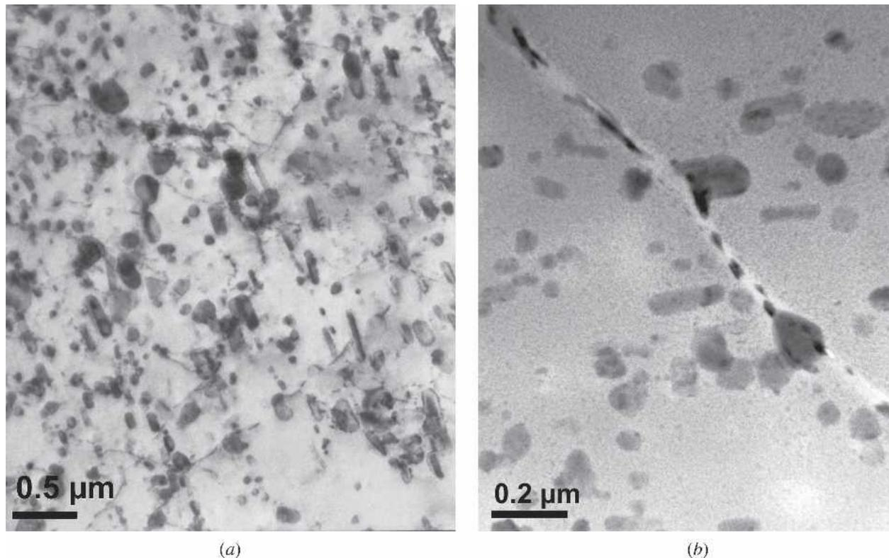
Fig. 9—TEM micrographs showing (a)  $\text{Mg}(\text{Zn}_2, \text{AlCu})$  and  $\text{Mg}_{32}(\text{Al}, \text{Zn})_{49}$ , in the as-received Al 7075-T6 sheet, and (b)  $\text{MgZn}_2$  particles at the grain boundary in the precipitation-free zone.
