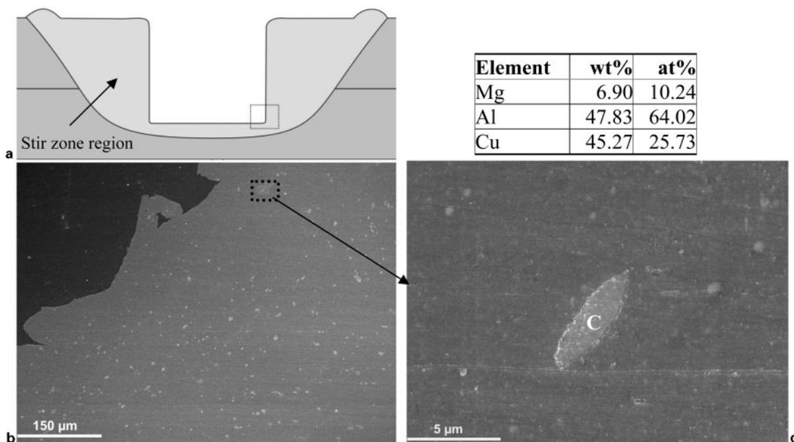
a schematic of location in stir zone of Al 2024 spot weld; b SEM image of location of melted S phase particle; c detail of melted S phase particle and EDX chemical analysis at location C
