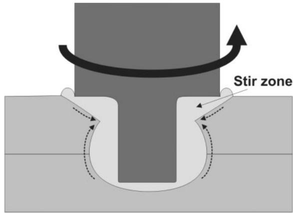
**5 Schematic representation showing material flow during friction stir spot welding, based on combination of particle tracer studies and numerical modelling:<sup>5</sup> flow of material causes S phase particles from as received Al 2024 material to be incorporated in stir zone**
