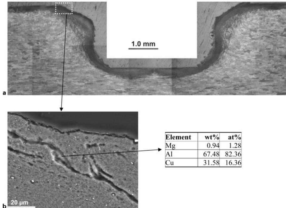
a optical micrograph of location in stir zone of Al 2024 spot weld; b SEM image of cracking
