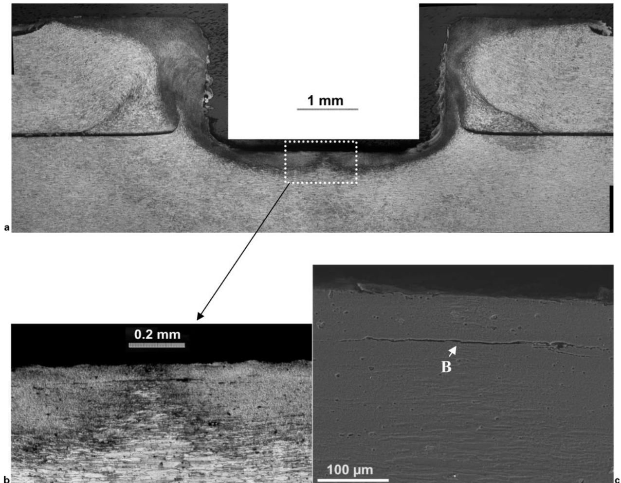
3 a optical micrograph of location, which exhibits cracking (in location beneath tip of rotating pin in rapidly quenched Al 7075 spot weld produced using plunge rate of  $10 \text{ mm s}^{-1}$  and dwell time of  $0.05 \text{ s}$ ), b optical micrograph of crack location and c SEM image of crack in detail: EDX analysis at location B was 73.1 wt-%Al, 20.2 wt-%Zn, 6.6 wt-%Cu
