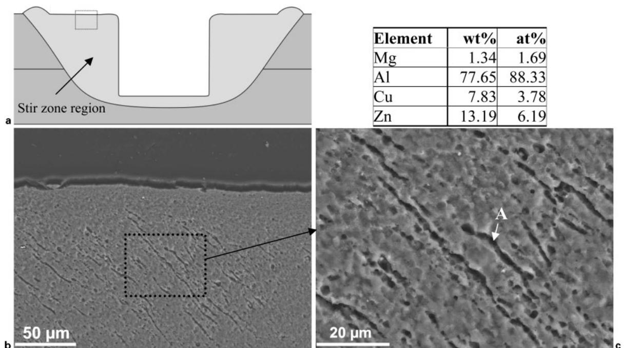
a schematic of location in Al 7075 spot weld stir zone; b SEM image of melted films; c detail of melted film and EDX chemical analysis at location A
