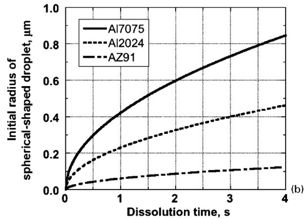
7 a phase diagram for pseudobinary showing locations of composition values used in equation (2) and b dissolution rate of melted eutectic films in stir zone region during 4 s long dwell period in Al 2024, Al 7075 and AZ91 friction stir spot welding
