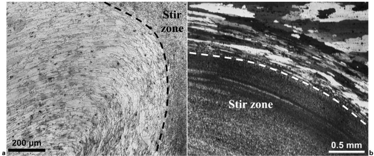
2 a optical micrograph showing transverse section through Al 7075 spot weld with grains in TMAZ elongated parallel to stir zone boundary (see dashed line) and b polarised light micrograph showing grains elongated parallel to shoulder periphery in TMAZ region (see dashed line) in horizontal cross-section through Al 7075 spot weld
