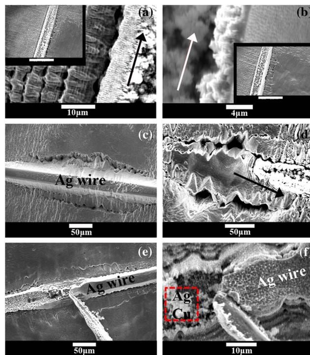
Fig. 3. (Color online) SEM images of the fs laser irradiated samples with mechanical clamping fixture: (a)  $0.08 \text{ J/cm}^2$ -3000 pulses, (b)  $0.08 \text{ J/cm}^2$ -4000 pulses, (c)  $0.08 \text{ J/cm}^2$ -6000 pulses, (d)  $0.08 \text{ J/cm}^2$ -10,000 pulses, and (e), (f)  $0.15 \text{ J/cm}^2$ -1000 pulses. The scale bar in the inset figures is  $100 \mu\text{m}$ , and the arrows show the location and direction of the Ag microwire, which was removed.
