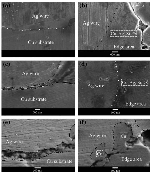
Fig. 5. Cross-sectional morphologies of the contact area (left) and edge area (right) in the samples irradiated at fluence of  $1.02 \text{ J/cm}^2$  with different pulse numbers: (a), (b) 500 pulses; (c), (d) 1000 pulses; and (e), (f) 2000 pulses.
