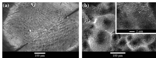
Fig. 8. SEM morphologies of the damaged cover glass: (a) general view and (b) craters and ripples.
