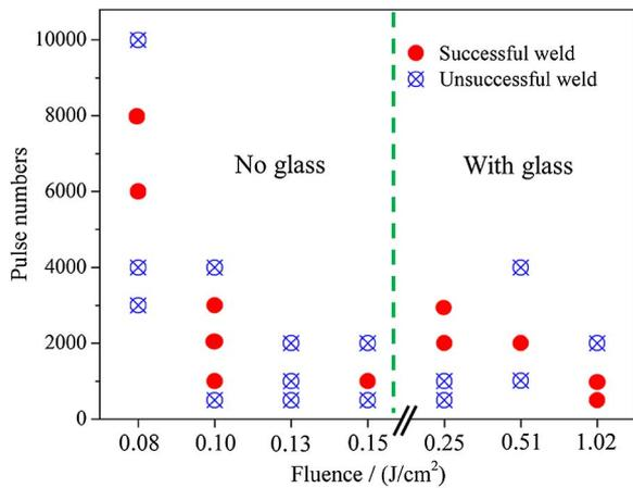
Fig. 4. (Color online) Summary of fs laser-induced microwelding of Ag microwire and Cu substrate.
