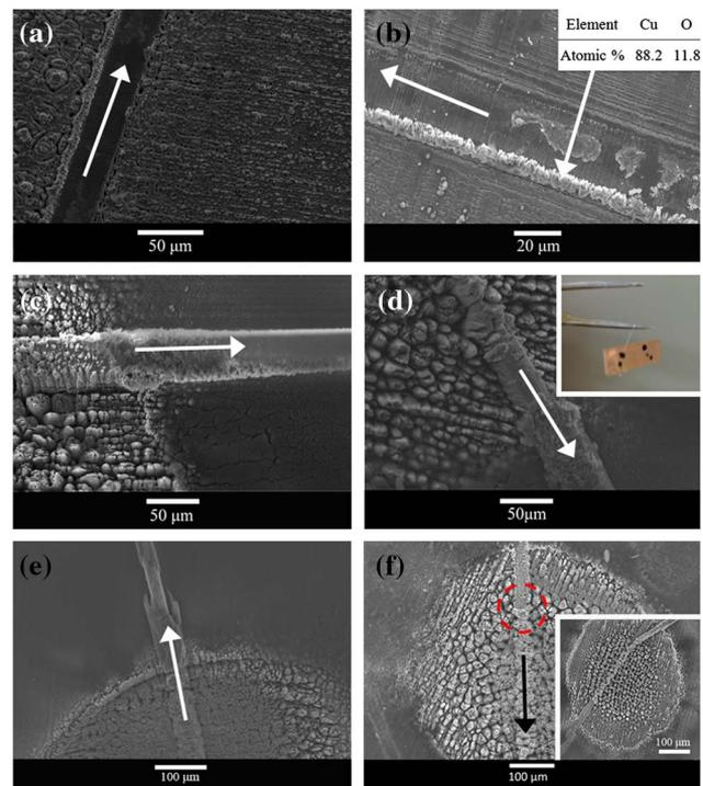
Fig. 2. (Color online) SEM images and EDS results of fs laser irradiated samples with glass–tape fixture: (a)  $0.25 \text{ J/cm}^2$ -500 pulses, (b)  $0.25 \text{ J/cm}^2$ -1000 pulses, (c)  $0.25 \text{ J/cm}^2$ -2000 pulses, (d)  $0.25 \text{ J/cm}^2$ -3000 pulses, (e)  $1.02 \text{ J/cm}^2$ -1000 pulses, and (f)  $1.02 \text{ J/cm}^2$ -2000 pulses. The arrows show the position and direction of the Ag microwire.
