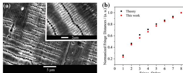
Fig. 7. (Color online) SEM morphologies of Cu substrate irradiated by 1000 laser pulse irradiation at a fluence of  $0.25 \text{ J/cm}^2$ : (a) periodical grooves and microholes and (b) comparison of experimental and calculated Fresnel diffraction pattern.
