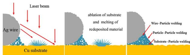
Fig. 6. (Color online) Schematic of fs laser microwelding process.
