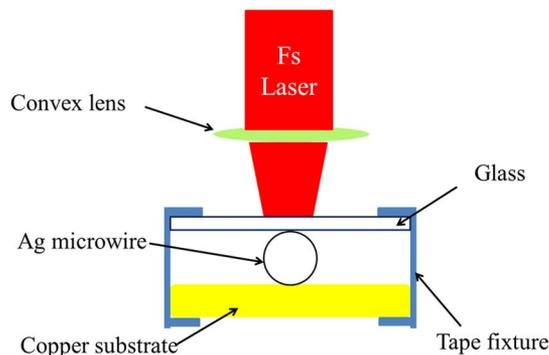
Fig. 1. (Color online) Schematic of fs laser microwelding experimental.
