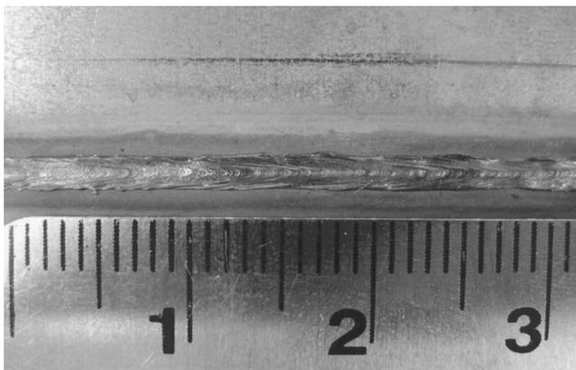
FIG. 10. Surface appearance of a diode laser lap weld on 1.0 mm galvanized steel sheets (GA45–45g/m<sup>2</sup> zinc coating) precoated with 70 μm thickness of Al by cold spray before welding. Welding speed was 0.7 m/min.
