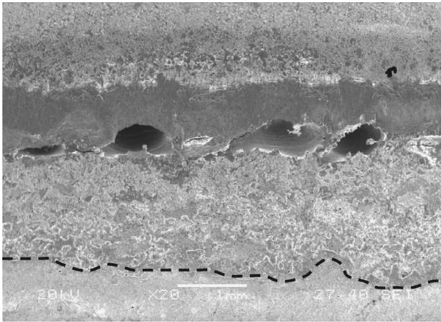
FIG. 6. Typical interfacial shear fracture appearance of weldments similar to that shown in Fig. 5, but without addition of Al to suppress Zn vapor evolution. The outlined area beside the weld has had its galvanneal coating removed by evaporation of the Zn. Welding speed 0.7 m/min.
