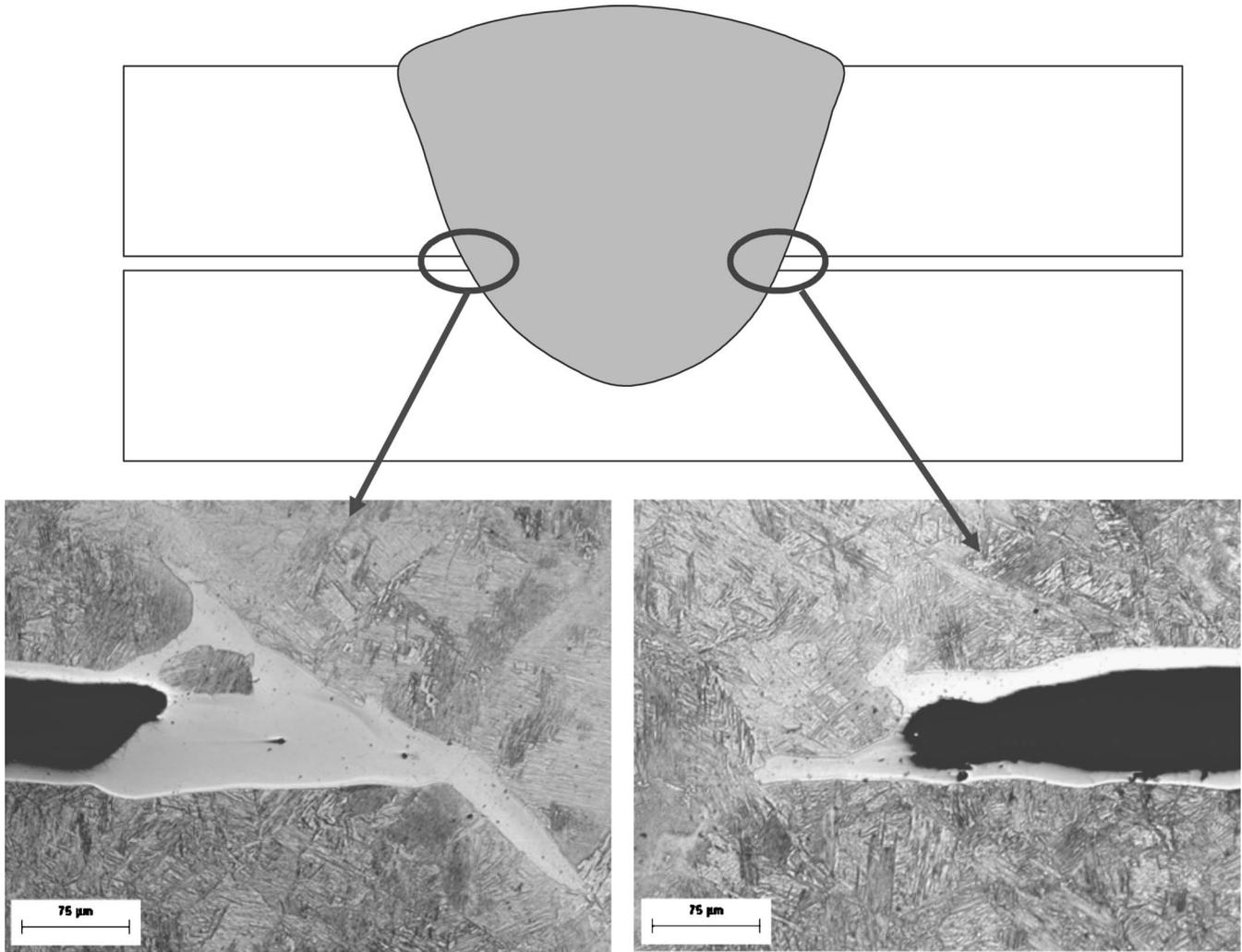
FIG. 9. High-magnification views of the crevice—weld fusion zone intersection regions of a diode laser weld made at 0.7 m/min, showing the solidified high-Al liquid films.
