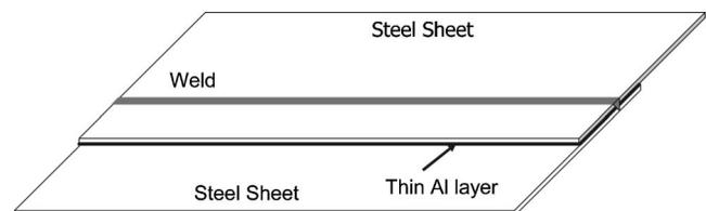
FIG. 1. Schematic diagram of weld coupon assembly for lap welding.
