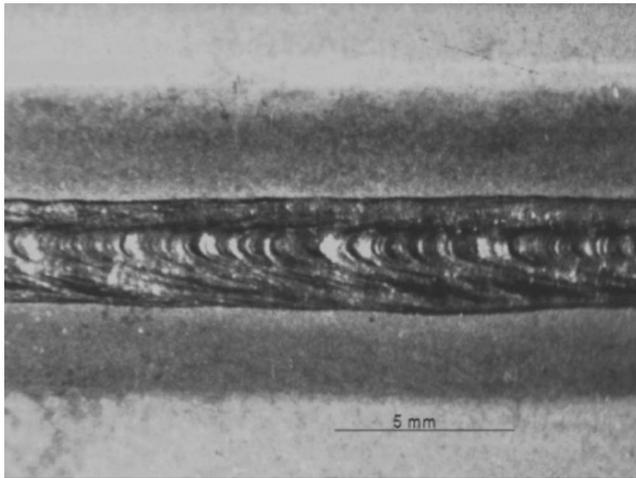
FIG. 2. Surface appearance of a lap weld on 1.0 mm galvanized steel, made with a 4 kW diode laser, welding speed 0.7 m/min, with 25  $\mu\text{m}$  Al foil inserted between tightly clamped sheets.
