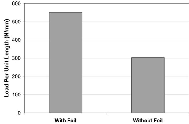
FIG. 4. Results (averages of three samples) of shear testing of diode laser lap welds made on tightly clamped 1-mm-thick DP600 galvanized steel sheets, with and without 25  $\mu\text{m}$  Al foil inserted between sheets.
