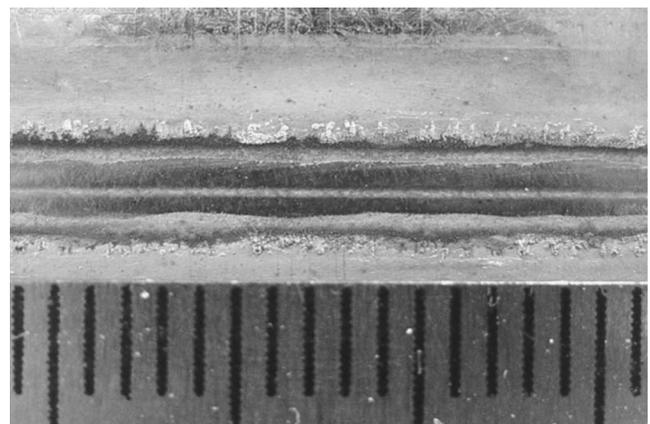
FIG. 11. Surface appearance of a diode laser lap weld on Al spray coated steel sheets, similar to Fig. 10 except 1.1 mm hot dip galvanized sheets with G170–70 g/m<sup>2</sup> zinc coating. Welding speed was 0.55 m/min.
