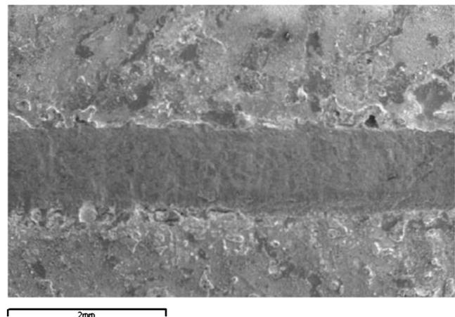
FIG. 5. Typical interfacial shear fracture appearance of diode laser lap welds made on 1-mm-thick galvanized coated DP600 steel with Al foil clamped between sheets. Welding speed was 0.7 m/min.
