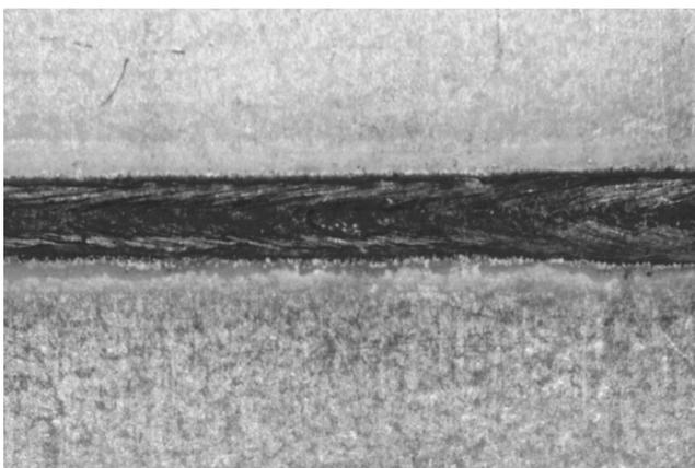
FIG. 7. Surface appearance of a lap weld made on 1.0 mm galvannealed steel using a 3 kW Nd:YAG laser, welding speed 5.0 m/min, with 50  $\mu\text{m}$  Al foil inserted between the sheets.
