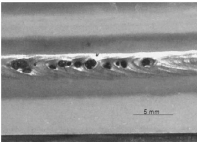
FIG. 3. Surface of a lap weld similar to that shown in Fig. 2 except without Al foil. Typical severe porosity due to zinc vapor evolution is visible.
