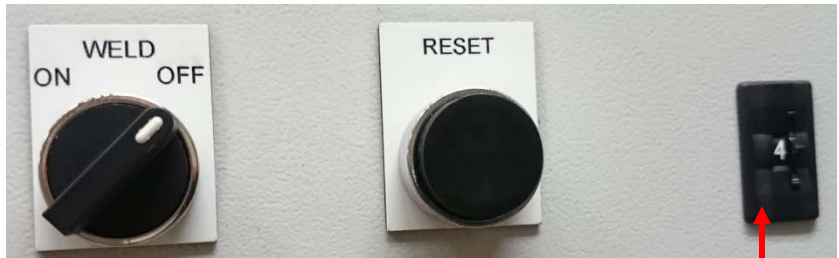
Switch lever • Showing "OFF" position • Turn clockwise (90 degrees downward) to switch "ON"
