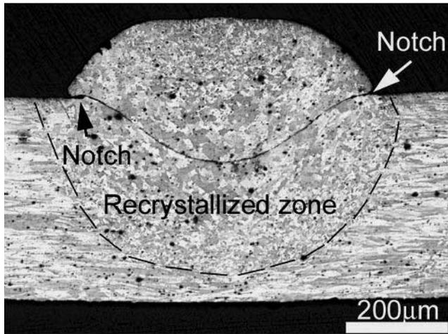
Fig. 13—OM cross-sectional micrograph of the joint between bare Ni wires welded at 400 A for 80 ms, showing solid-state bonding at the interface as well as the presence of a sharp notch at the edge of the joint and more deformation of Ni wires compared with the Au-plated Ni wires joint (Fig. 3(d1)).
