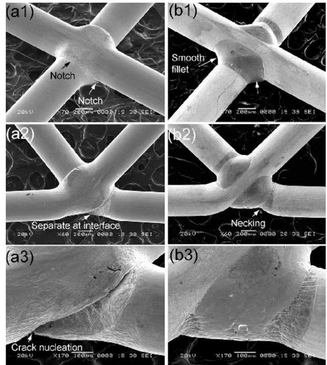
Fig. 15—SEM images of (a) joints between Au-plated Ni wires and (b) joints between bare Ni wires welded at 600 A for 1 ms (1: as-welded joints, 2: after loading, and 3: details of the necking region or the interface region).
