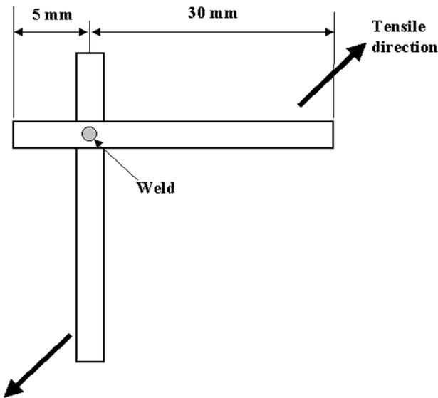
Fig. 1—Schematic illustrations of the cross-wire joint assembly and loading in tensile-shear testing.
