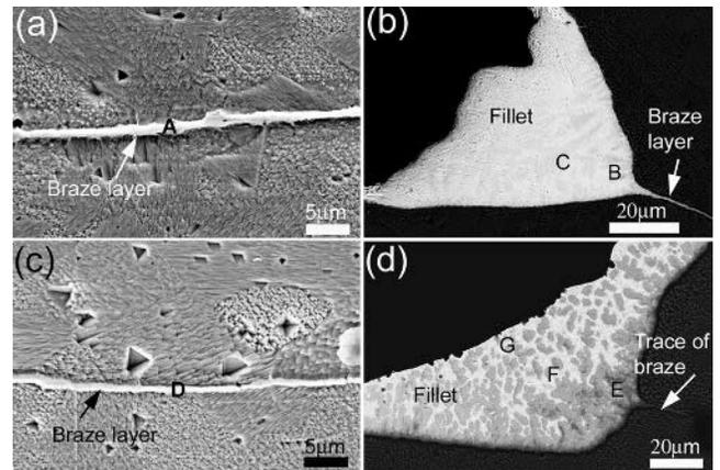
Fig. 5—SEM cross-sectional images of the (a) interface and (b) fillet in the joint welded at 250 A for 80 ms as well as the (c) interface and (d) fillet in the joint welded at 400 A for 80 ms. (The compositions of different regions are listed in Table I).
