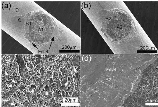
Fig. 9—SEM fractographs obtained from the joint welded at 350 A for 1 ms after the tensile-shear test: (a) low magnification of a wire, (b) opposite wire, (c) details of region A in (a), and (d) details of region B2 in (b). (The compositions of different regions are listed in Table II).
