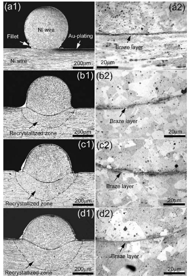
Fig. 4—OM cross-sectional micrographs of joints between Au-plated Ni wires welded at 350 A for (a1) and (a2) 1 ms, (b1) and (b2) 10 ms, (c1) and (c2) 40 ms, and (d1) and (d2) 80 ms. ((a2) through (d2)) show detailed center interfacial regions in (a1) through (d1), respectively.
