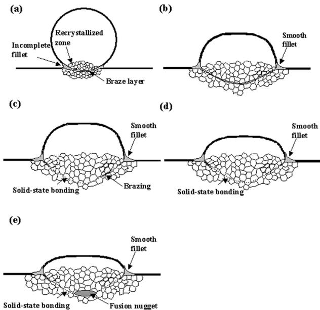
Fig. 11—Schematic illustration of joint formation during RMW of Au-plated Ni wires: (a) brazing at low welding current with the formation of incomplete fillet, (b) brazing at high welding current with the formation of smooth fillet and increased Ni content within braze layer, (c) combinations of brazing and solid-state bonding at the interface, (d) solid-state bonding, and (e) combinations of solid-state bonding and fusion welding.
