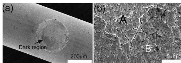
Fig. 8—SEM fractographs obtained from the joint welded at 300 A for 1 ms after tensile-shear test, showing (a) interfacial fracture between the wires and (b) occasional local bonding (area A) between Au plating corresponding to the dark region in (a); area B represents a micrograph of the original Au-plating surface.
