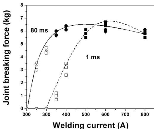
Fig. 6—Effect of welding current on the breaking force for 1 and 80 ms weld times (open and closed symbols indicate fracture at interface between wires and in the HAZ of Ni wire, respectively).
