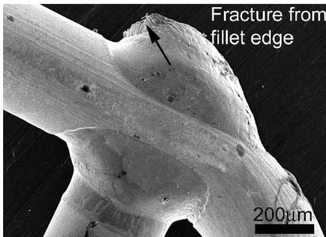
Fig. 10—SEM image showing fracture occurring in the HAZ from the edge of the fillet in the Au-plated Ni wires joint welded at 600 A for 1 ms.
