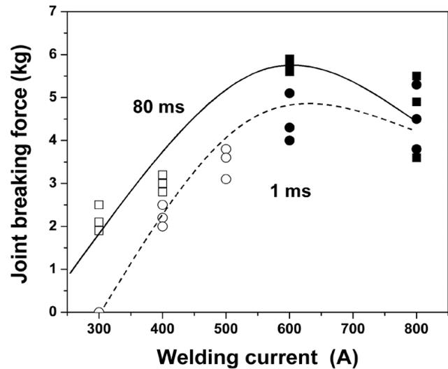
Fig. 12—Effect of welding current on breaking force of joints between bare Ni wires welded with 1 and 80 ms hold time (open and closed symbols indicate fracture at interface between wires and in the HAZ of Ni wire, respectively).
