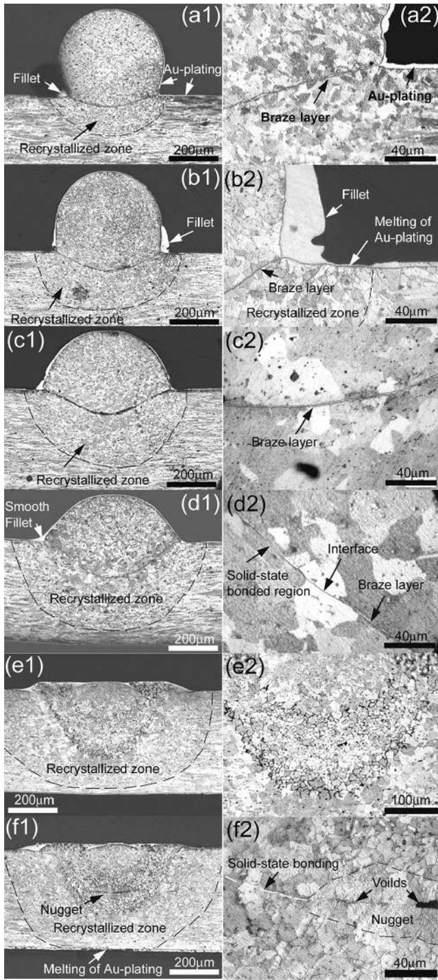
Fig. 3—OM cross-sectional micrographs of joints between Au-plated Ni wires welded at (a1) and (a2) 250 A, (b1) and (b2) 300 A, (c1) and (c2) 350 A, (d1) and (d2) 400 A, (e1) and (e2) 600 A, and (f1) and (f2) 800 A for the welding time of 80 ms. ((a2) through (f2)) show detailed regions of either the fillet or the interface in (a1) through (f1), respectively.
