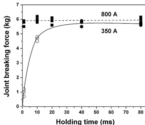
Fig. 7—Effect of the hold time on the breaking force of joints welded at 350 and 800 A (open and closed symbols indicate fracture at interface between wires and in HAZ of Ni wire, respectively).
