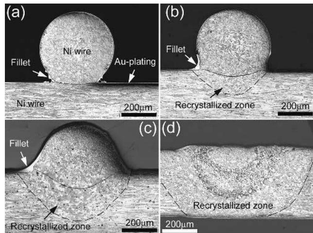
Fig. 2—OM cross-sectional micrographs of joints between Au-plated Ni wires welded at (a) 350 A, (b) 400 A, (c) 600 A, and (d) 800 A for welding time of 1 ms. (The boundaries of the recrystallized zone are indicated by dashed lines).
