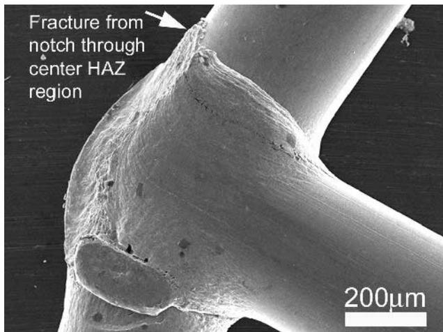
Fig. 14—SEM images showing HAZ fracture occurring from the root of the joint between the bare Ni wires through the center region of the HAZ (welded at 600 A for 1 ms).
