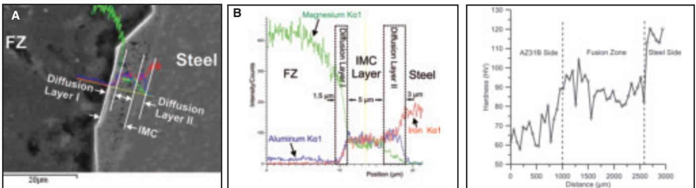
Fig. 10 — EDS composition line scans at the FZ/steel interface: A — SEM image of the interface; B — line scans of Al, Fe, and Mg.
