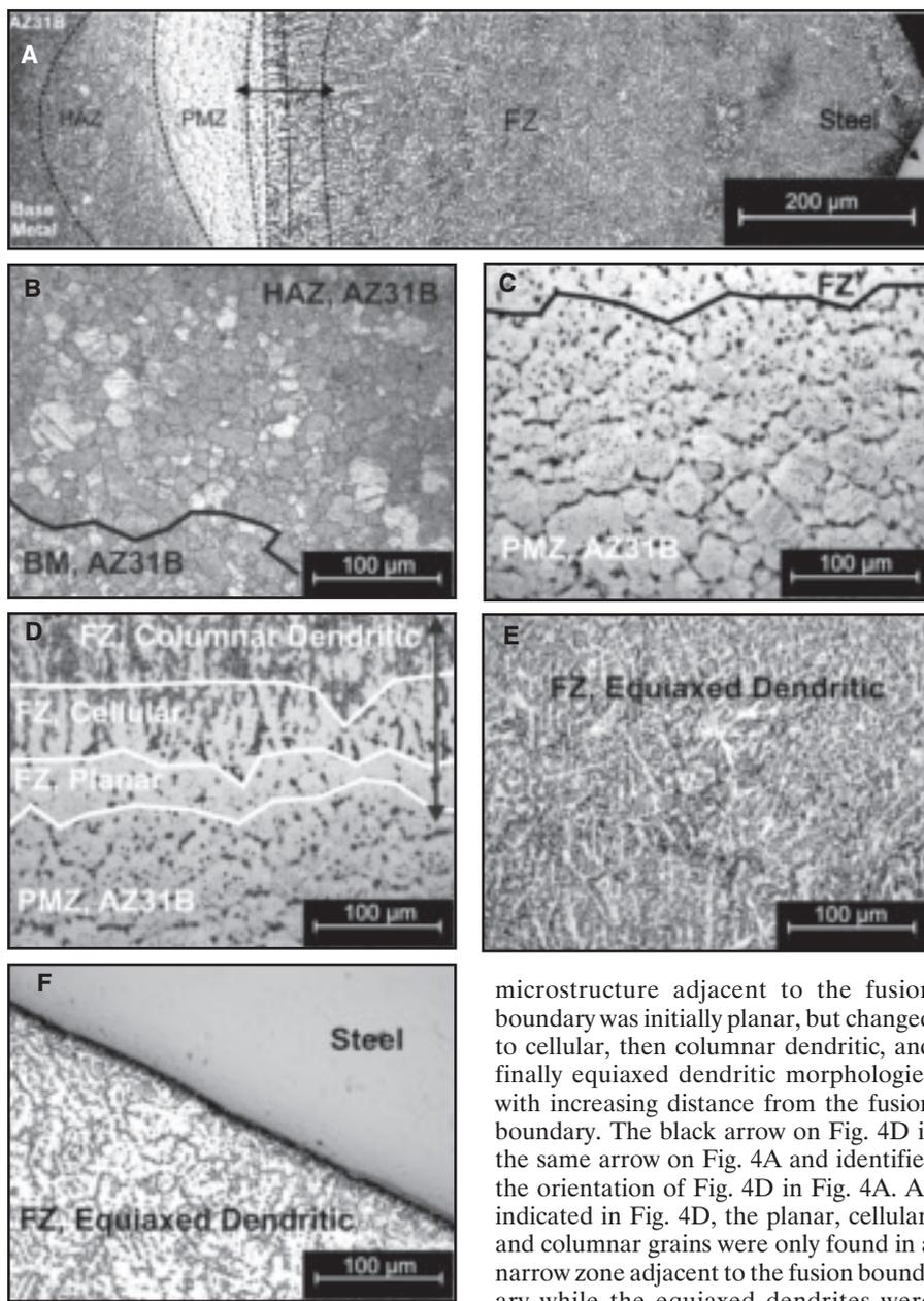
Fig. 4 — Photomicrographs of different microstructural regions in the laser brazed AZ31B/steel joint.
