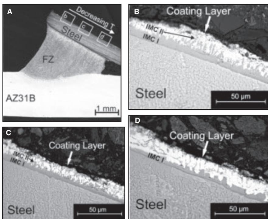
Fig. 6 — Thickness and morphology variation of IMC layer in different positions of the steel/coating layer interface indicated in the following: A, B — Upper; C — middle; D — bottom part of the joint.
