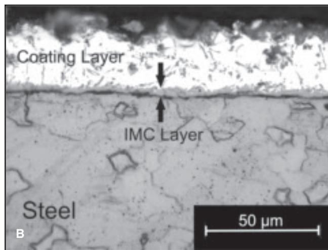
Fig. 1 — Transverse section of original steel sheet showing: A — The Al-12Si coating layer; B — the preexisting Fe-Al-Si IMC layer at the steel/coating layer interface.
