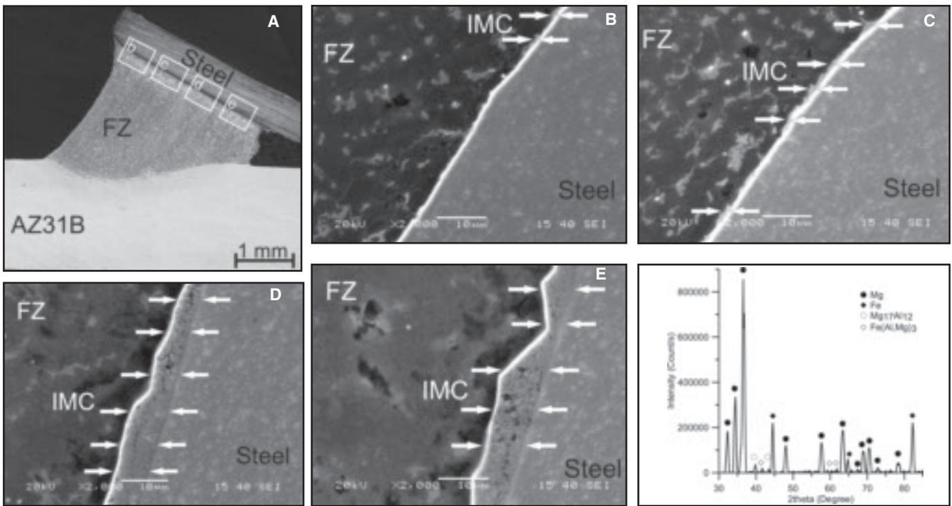
Fig. 8 — A — SEM images in different positions of the steel/FZ interface; B–E — IMC layer in b–e zones shown in A.
