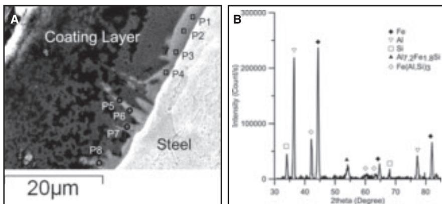
Fig. 7 — Al-12Si coating layer-steel interface of a laser brazed AZ31B-steel joint: A — SEM image of IMC layer along interface demonstrates locations with EDS analysis; B — X-ray diffraction pattern of the interface.
