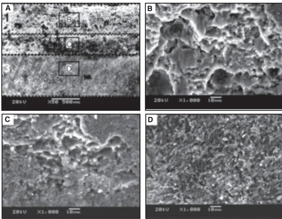
Fig. 13 — SEM images of typical fracture surface of fusion zone side after tensile shear test. A — Fusion zone side including the following: B — top of the surface indicated by B; C — middle of the surface indicated by C; D — bottom of the surface indicated by D.
