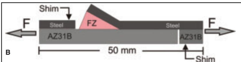
Fig. 2 — A — Schematic of the laser brazing system used for joining the AZ31B Mg and aluminum-coated steel sheets in the single flare bevel lap joint configuration; B — schematic of the 5-mm-wide tensile shear test specimens.
