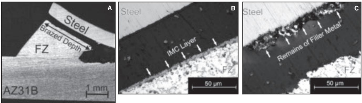
Fig. 12 — Fracture location of the tensile shear test specimen. A — Fractured specimen; B — crack propagation in bottom of the joint; C — crack propagation in upper part of the joint.
