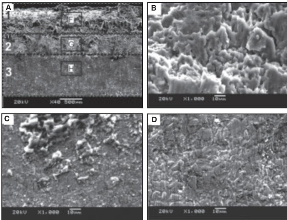
Fig. 14 — SEM images of typical fracture surface of steel side after tensile shear test. A — Steel side including: B — top of the surface indicated by F; C — middle of the surface indicated by G; D — bottom of the surface indicated by H.
