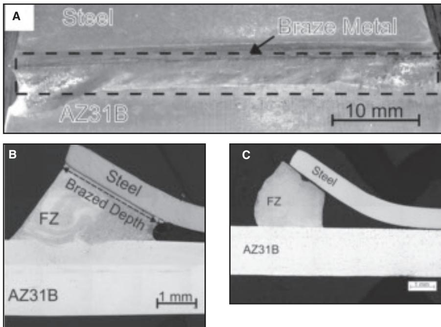
*Fig. 3 — Laser brazed AZ31B-to-steel sheets made using 8 mm/s travel speed and 2.2 kW laser beam power: A — Top bead; B — transverse section of a brazed Al-12Si coating steel; C — transverse section of a brazed uncoated steel sheet.*
