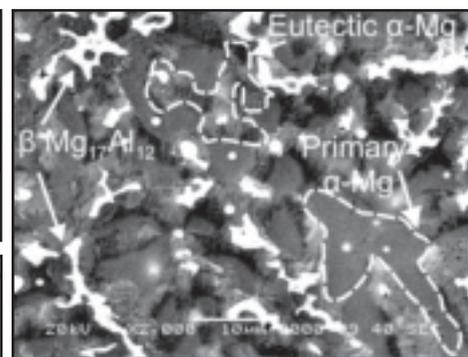
Fig. 5 — SEM image of the fusion zone microstructure shows primary and eutectic α-Mg with divorced eutectic β-phase in interdendritic regions.
