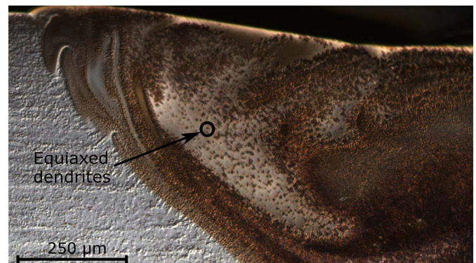
Fig. 8. Close-up of the region where dendrite fragmentation into a CuAlMn base material-like composition region occurred. The circle represents a region analysed in Fig. 7 showing the equiaxed dendrites.
