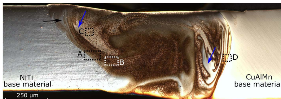
Fig. 3. Macrograph of the NiTi/CuAlMn dissimilar laser joint. Regions A to D are analysed separately. The black and blues arrows indicate regions where macrosegregation occurred: black for NiTi and blue for CuAlMn. (For interpretation of the references to colour in this figure legend, the reader is referred to the web version of this article.)
