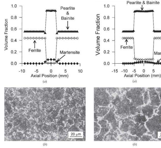
Fig. 18-Results of a friction weld made using the optimal welding condition: (a) predicted volume fraction of ferrite, martensite, pearlite, bainite; and (b) photomicrograph showing ferrite (white) and fine pearlite, bainite, and martensite (gray) at the weld interface and on the center line.
