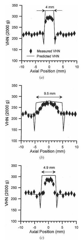
Fig. 21—The measured and predicted microhardness (VHN) vs axial position along the center line of welds made using (*a*) optimal, (*b*) long-time, and (*c*) hard and fast welding conditions.
