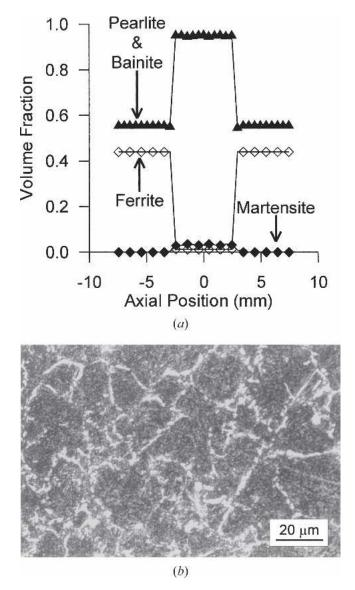
Fig. 20—Results of a friction weld made using the hard and fast welding condition: (*a*) predicted volume fractions of ferrite, pearlite, bainite, and martensite; and (*b*) photomicrograph showing ferrite (white) and fine pearlite, bainite, and martensite (gray) at the weld interface and on the center line.
