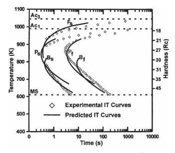
Fig. 16—Experimental IT curves for AISI/SAE 1045 steel<sup>[32]</sup> and transformation times predicted using Kirkaldy *et al.*'s<sup>[15,16,17]</sup> modified microstructure evolution model.
