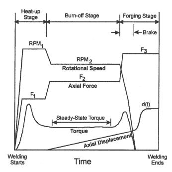
Fig. 3—The normal variations of the predefined rotational speeds and axial forces and the resultant torque and axial displacement during direct-drive friction welding.
