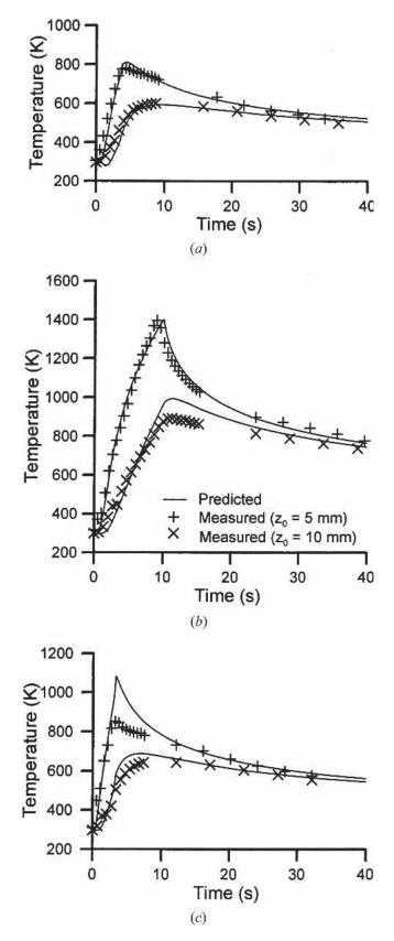
Fig. 14—The predicted and measured center line temperatures from embedded thermocouples originally placed at the center line and  $z_0 = 5$  mm and  $z_0 = 10$  mm from the weld interface of AISI/SAE 1045 steel friction welds made using (*a*) optimal, (*b*) long-time, and (*c*) hard and fast welding condition.
