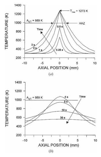
Fig. 13—Displacement-compensated predicted temperatures vs axial position along the center line of a weld made using the optimal welding conditions: (*a*) during the heating and burn-off stages and (*b*) during the forging and cooling stages.
