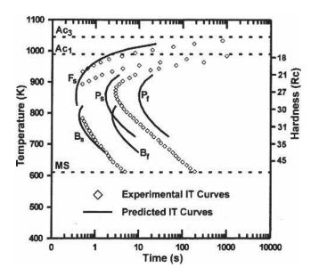
Fig. 15—Experimental IT curves for AISI/SAE 1045 steel<sup>[32]</sup> and transformation times predicted using Kirkaldy *et al.*'s<sup>[15,16,17]</sup> original microstructure evolution model.
