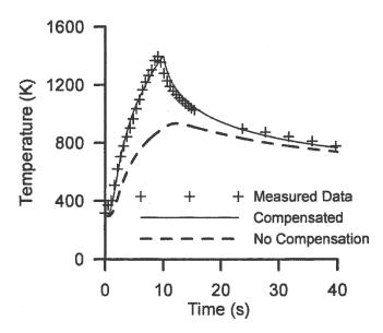
Fig. 12—The effect of compensating for the axial displacement of the weld specimen and thermocouple with respect to the weld interface on the measured and predicted temperatures *vs* time for the long-time welding condition.
