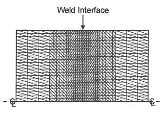
Fig. 6—A typical finite-element graded mesh used, which consists of 1496 triangular, toroidal elements.
