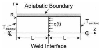
Fig. 5—The geometric domain and the boundary conditions used in the transient thermal model.
