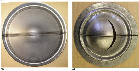
Fig. 8 Dome tested specimens. (a) Parent metal of DP980. (b) Details of crack in (a). (c) Welded specimen of DP980 at welding speed of 1.3 m/min. (d) Details of crack in (c). (e) Parent metal of HSLA. (f) Welded specimen of HSLA.
