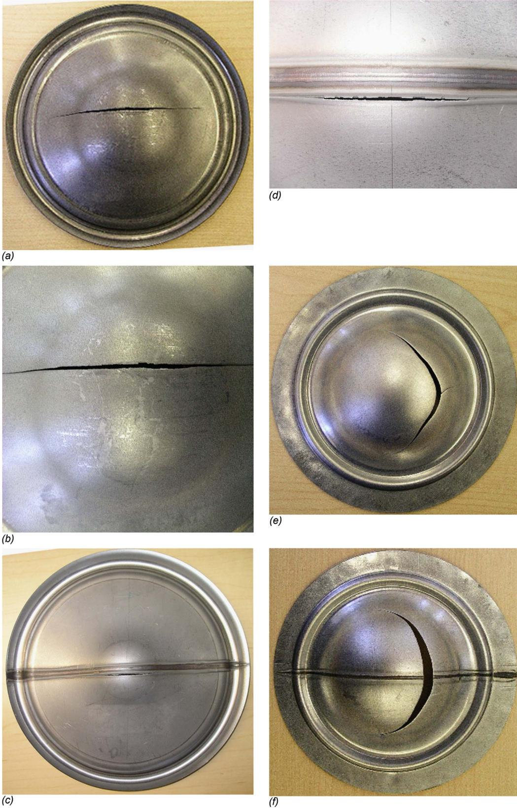
**Fig. 8** Dome tested specimens. (a) Parent metal of DP980. (b) Details of crack in (a). (c) Welded specimen of DP980 at welding speed of 1.3 m/min. (d) Details of crack in (c). (e) Parent metal of HSLA. (f) Welded specimen of HSLA.
