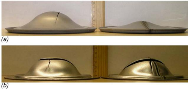
**Fig. 9** Side views of dome tested samples. The dome heights of the parent metal and welded specimen are 30.4 and 13.2 mm for DP980 (a), and 32.5 and 31.8 mm for HSLA (b). Welding speed is 1.6 m/min and welding direction is parallel to the rolling direction.
