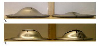
Fig. 9 Side views of dome tested samples. The dome heights of the parent metal and welded specimen are 30.4 and 13.2 mm for DP980 (*a*), and 32.5 and 31.8 mm for HSLA (*b*). Welding speed is 1.6 m/min and welding direction is parallel to the rolling direction.
