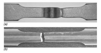
Fig. 7 Typical tensile tested DP welded specimens: (*a*) Transverse and (*b*) longitudinal
