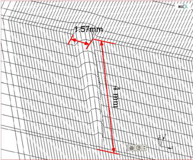
Fig. 2 – Mesh and dimensions for pre-assumed keyhole.
