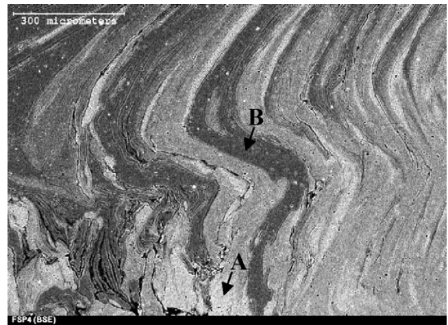
Fig. 4. SEM backscattered electron micrograph lamellae in the stir zone of seam weld produced using 2500 rpm and tool penetration of 0.24 mm. EDX analysis from location A was 86.2% Al, 9.5% Zn, 2.8% Cu, 1.5% Mg, and location B was 97.2% Al, 1.7% Cu, 0.6% Zn, 0.5% Mg, all in wt%.
