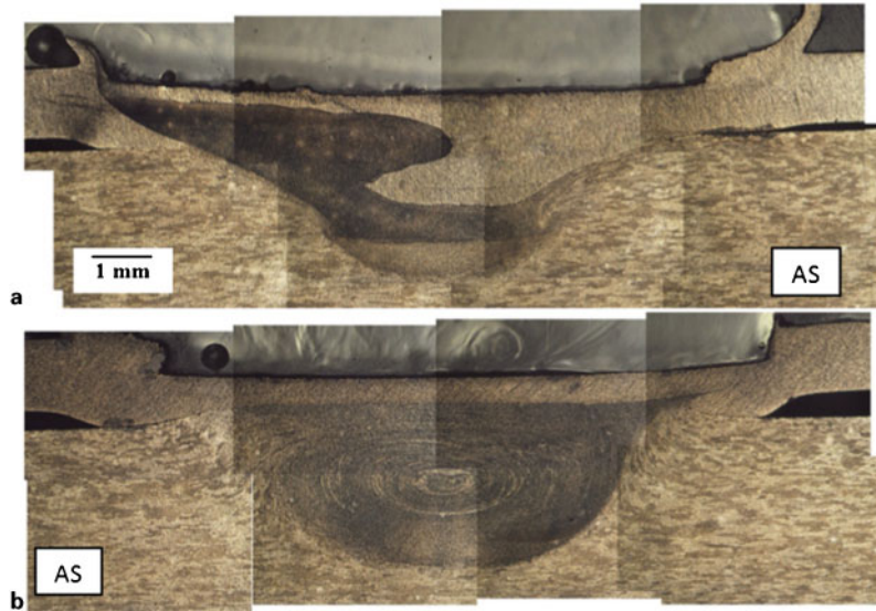
8 Lap weld produced using tool with helical threads on pin when tool rotation is in a clockwise (transferring material downwards) and b counterclockwise (promoting material movement upwards)
