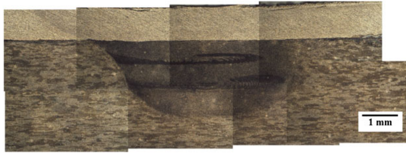
3 Lap weld produced using groove tool at 88 \text{ mm min}^{-1}
