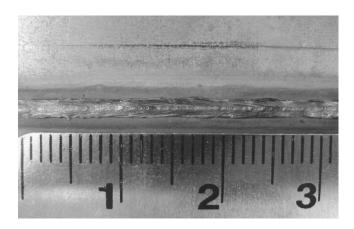
FIG. 10. Surface appearance of a diode laser lap weld on 1.0 mm galvannealed steel sheets (GA45–45g/m<sup>2</sup> zinc coating) precoated with 70  $\mu$ m thickness of Al by cold spray before welding. Welding speed was 0.7 m/min.
