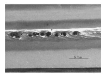
FIG. 3. Surface of a lap weld similar to that shown in Fig. 2 except without Al foil. Typical severe porosity due to zinc vapor evolution is visible.
