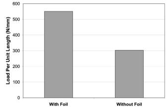
FIG. 4. Results (averages of three samples) of shear testing of diode laser lap welds made on tightly clamped 1-mm-thick DP600 galvannealed steel sheets, with and without 25  $\mu$ m Al foil inserted between sheets.
