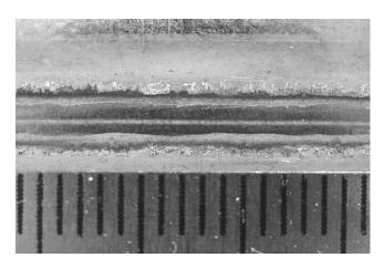
FIG. 11. Surface appearance of a diode laser lap weld on Al spray coated steel sheets, similar to Fig. 10 except 1.1 mm hot dip galvanized sheets with G170–70 g/m<sup>2</sup> zinc coating. Welding speed was 0.55 m/min.
