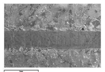
FIG. 5. Typical interfacial shear fracture appearance of diode laser lap welds made on 1-mm-thick galvanneal coated DP600 steel with Al foil clamped between sheets. Welding speed was 0.7 m/min.
