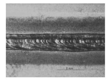
FIG. 2. Surface appearance of a lap weld on 1.0 mm galvannealed steel, made with a 4 kW diode laser, welding speed 0.7 m/min, with 25  $\mu$ m Al foil inserted between tightly clamped sheets.
