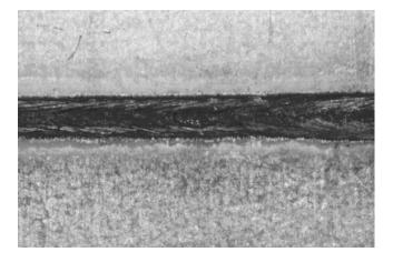
FIG. 7. Surface appearance of a lap weld made on 1.0 mm galvannealed steel using a 3 kW Nd:YAG laser, welding speed 5.0 m/min, with 50  $\mu$ m Al foil inserted between the sheets.
