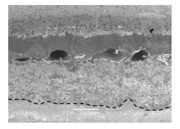
FIG. 6. Typical interfacial shear fracture appearance of weldments similar to that shown in Fig. 5, but without addition of Al to suppress Zn vapor evolution. The outlined area beside the weld has had its galvanneal coating removed by evaporation of the Zn. Welding speed 0.7 m/min.
