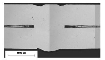
FIG. 8. Transverse cross-sectional view of the lap weld illustrated in Fig. 7, showing freedom from vapor-induced defects.
