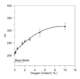
Figure 5 Weld hardness versus oxygen content in argon shielding gas.
