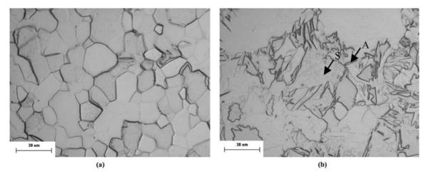
Figure 2 Cross sections of (a) base metal and (b) weld made with pure argon shielding gas.
