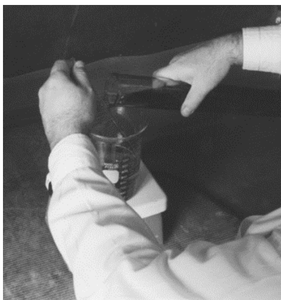
Fig. 1 Magnetic stirring plate with a magnetic bar for stirring, for use when mixing etchants. Slowly add the liquid ingredients to the solvent by dripping them down a glass stirring rod. If the solution is more dangerous than this one, wear protective gloves and use a face shield. If mixing generates substantial heat, it is a good practice to place a cooling jacket around the beaker.
