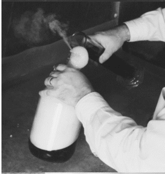
Fig. 2 Illustration of a bad mixing practice. The acid ingredient was poured into an empty acid bottle, and the solvents were added without stirring or cooling. The solution may erupt in the metallographer's face at any moment. It is essential to use gloves on at all times when handling chemicals. Consult the reference guide for the appropriate gloves for a given chemical, for example Nitrile are excellent for HCl and most other acids and solvents. However, if dealing with concentrated HNO 3 , and H 2 SO 4 then nitrile provide little to no resistance and PVC (vinyl) gloves are recommended.
