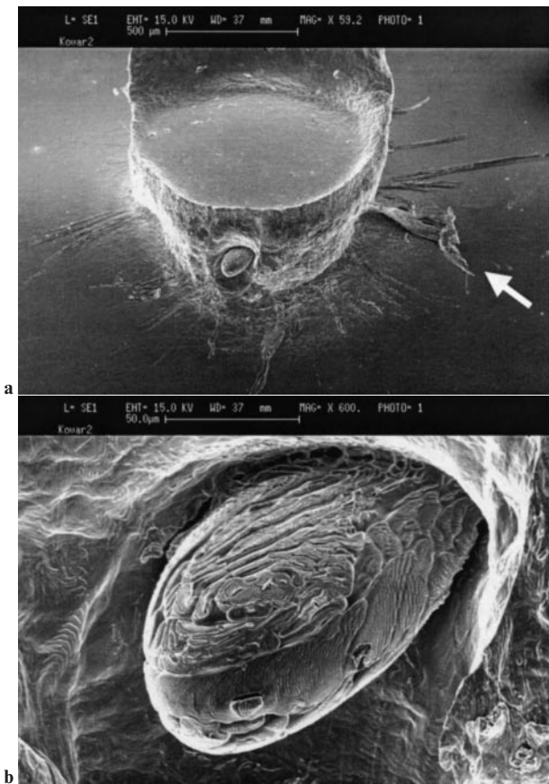
5 Weld metal expulsion (arrowed in a ): b shows detail of solidified molten metal being expelled from hole on pullout button in a (SEM)
