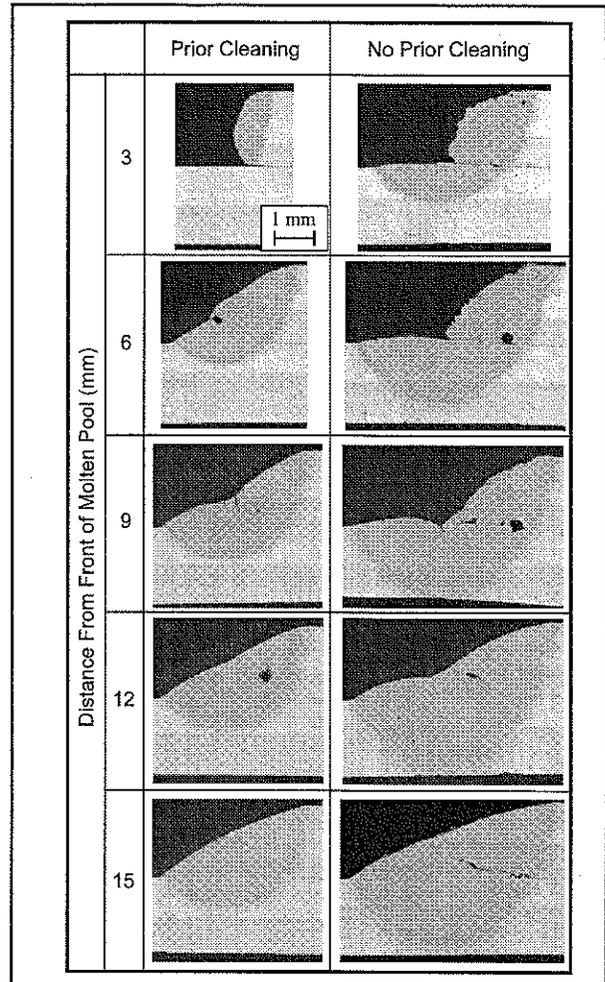
Fig. 16 — Cross sections through fillet weld in lap joints craters showing weld pool development, 1.5-mm-thick aluminum Alloy 5182 at 1 m/min.
