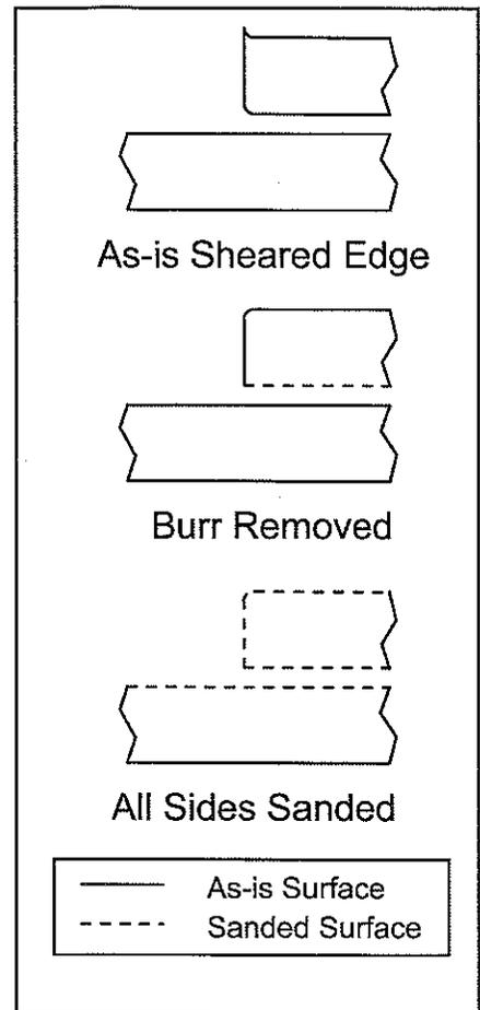
Fig. 4 — Sanding and cleaning conditions.
