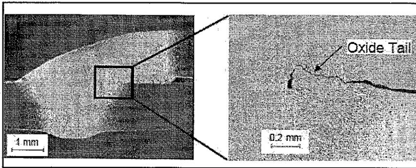
Fig. 3 — Fillet weld in lap-joint with insufficient clamping showing oxide tail defect. Travel speed 1 m/min.
