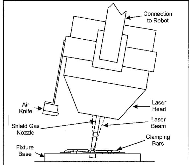
Fig. 2 — Diode laser welding fixture and shielding gas setup.
