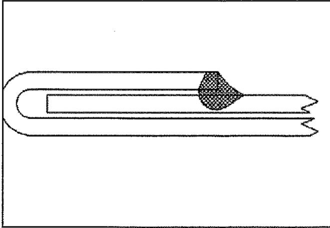
Fig. 1 — Cross section of in lap joints weld configuration.
