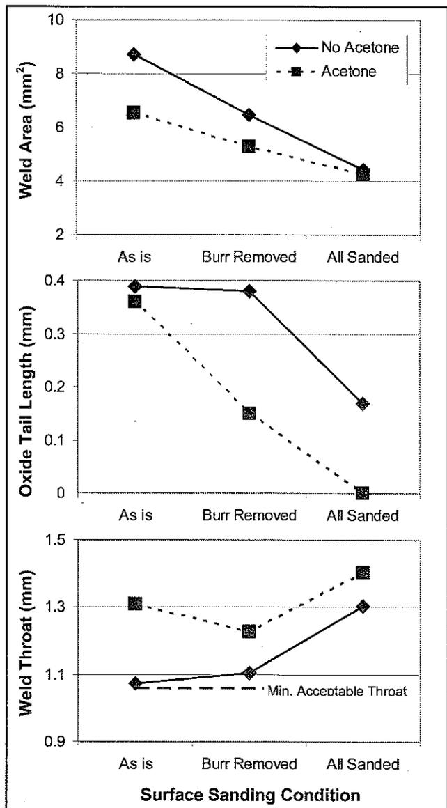
Fig. 6 — Effect of cleaning on weld cross-sectional area, oxide tail length, and weld throat. Fillet welds in lap joints on 1.5-mm-thick aluminum Alloy 5182 at 1 m/min.
