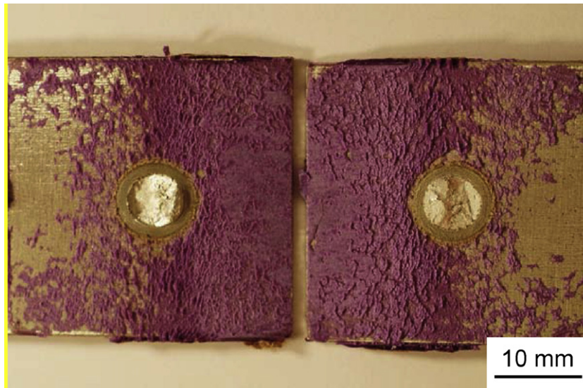
Fig. 2. A macroscopic image of a typical fatigue fracture surface of the WB Mg/Mg joint, showing the retained adhesive layer and the central fusion zone where the adhesive was squeezed or burned off.
