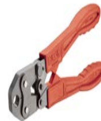
Traditional method of manually crimping pipes.
