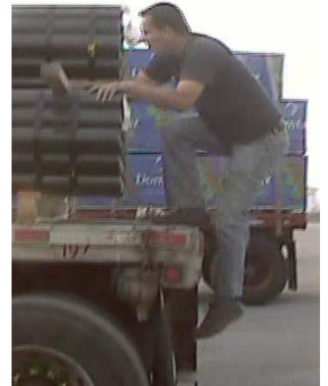
Getting on flatbed trailer using the rub rail and bumper for support
