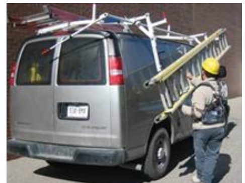
Storing ladder on a hydraulic drop down ladder rack
