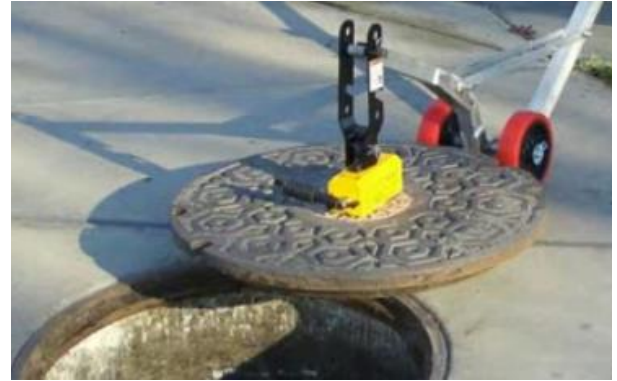
Magnetic hole cover lifter
