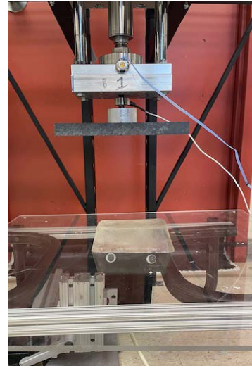
Figure 1: Experimental apparatus used for controlled mechanical loading, consisting of a linear actuator, specimen platform, and an ultrasound probe positioned below the specimen to measure subsurface deformation during loading.
