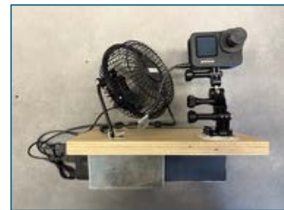
Figure 1: Custom wooden mount with GoPro camera, fan, and power pack.
