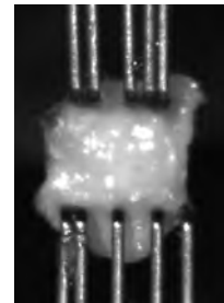
Figure 2: Single layer specimen mounted for tensile testing.
