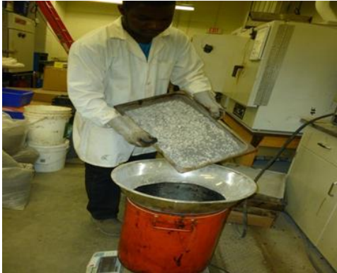
Placing batched virgin aggregate for mixing
