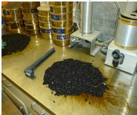
Determination of maximum relative density for conditioned mix in progress
