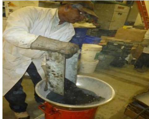
Placing batched 40% RAP aggregate for mixing
