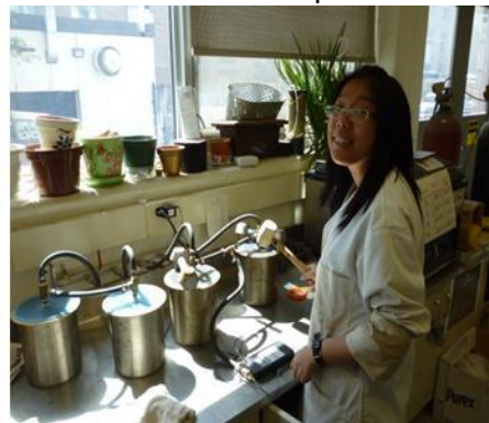
Determination of maximum relative density for conditioned mix in progress
