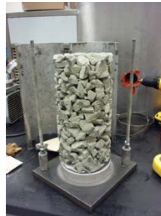
Compacted LWA sample ready to be transferred into the resilient modulus apparatus
