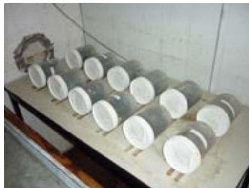
LWA samples undergoing freeze-thaw resistance testing
