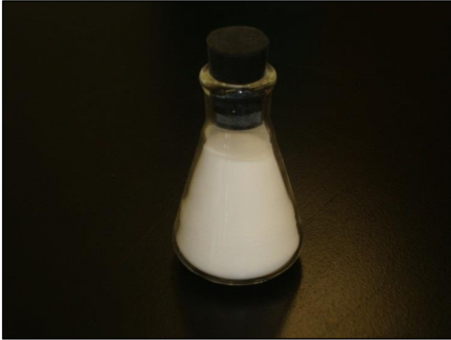
Nanosilica sample – particle size between 10 – 20 nanometers
