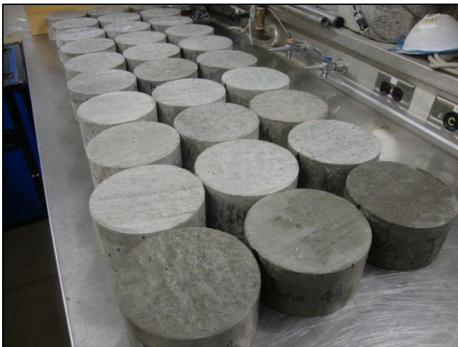
Laboratory samples for friction with British Pendulum Test and noise absorption with acoustical tube test
