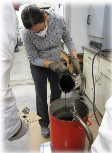
Xiomara Sanchez (PhD Candidate) adding asphalt cement during mixing process
