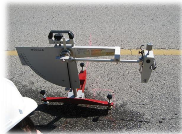
Friction testing using the British Pendulum
