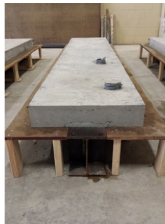
Cast-In-Place Slab Specimen (note girder)
