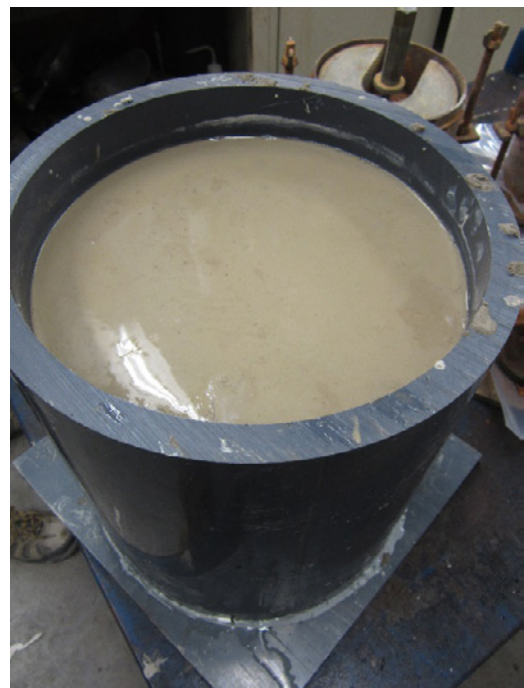
U-fill sample during bleeding test
