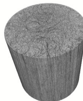
3D image of asphalt illustrates voids, aggregates and mastics
