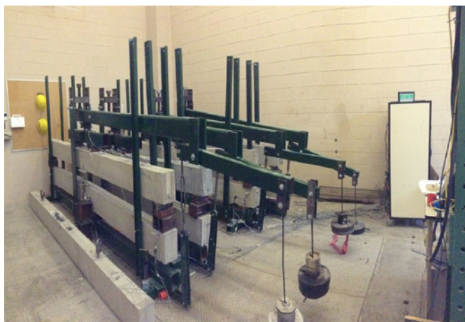
GFRP prestressed concrete beams subjected to sustained loads in mechanical loading frames
