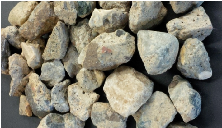
Recycled Concrete Aggregate
