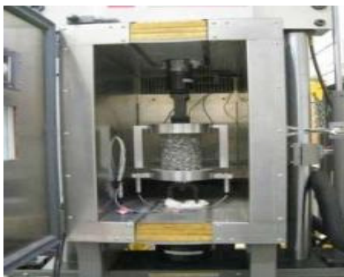
Dynamic modulus test setup
