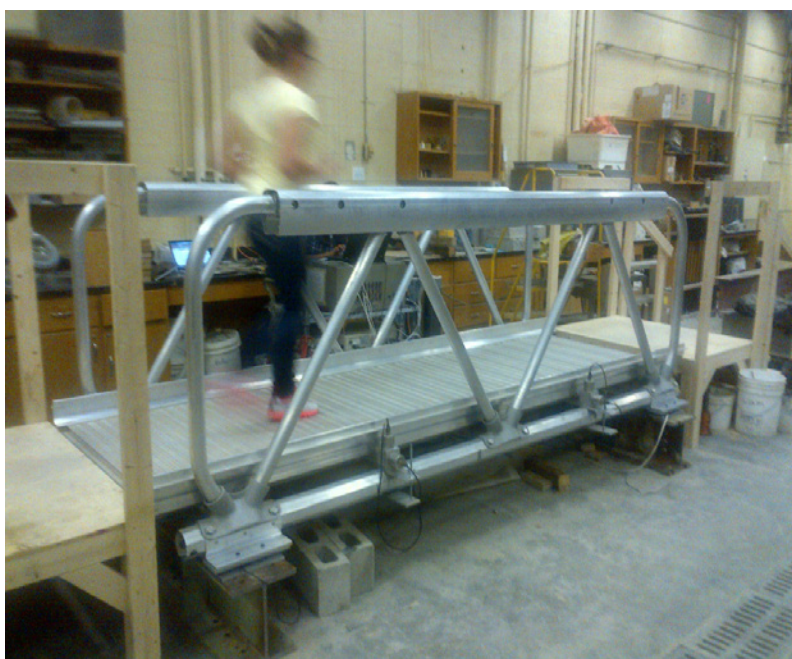
Running Test on Short Span Laboratory Specimen
