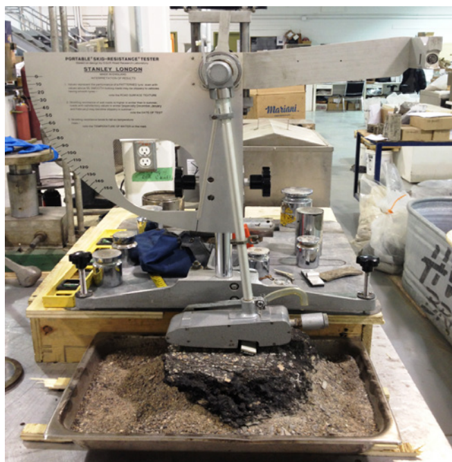
British Pendulum laboratory testing on samples of existing asphalt concrete from Kuujuaq airport
