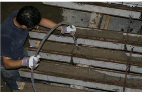
Casting of concrete beam specimens
