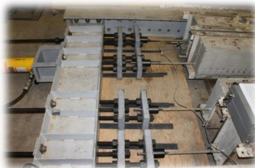
Prestressing bed for pretensioned beams
