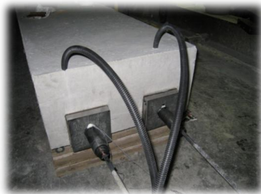
End of concrete beam showing prestressing anchor and tubes used for filling post-tensioning ducts with grout
