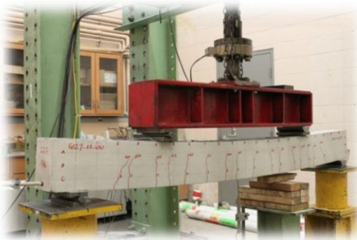
Cracked CFRP-pretensioned beam being testing to failure
