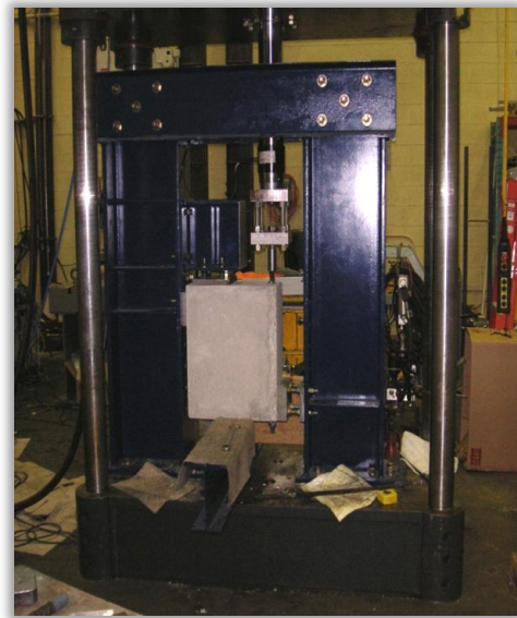
Test apparatus used to study effect of RCA on reinforcement bond to concrete
