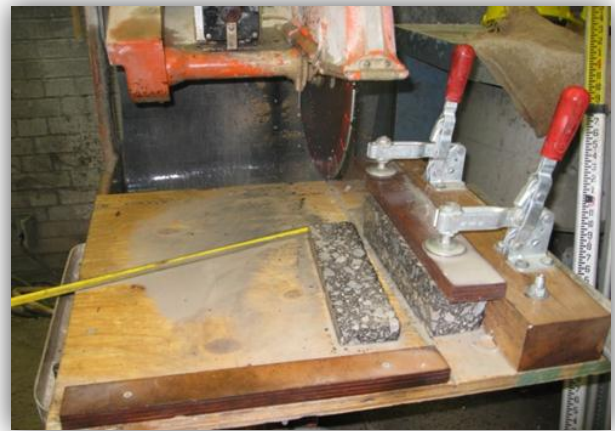
Preparing Hot Mix Asphalt containing Recycled Asphalt Shingles flexural fatigue beams
