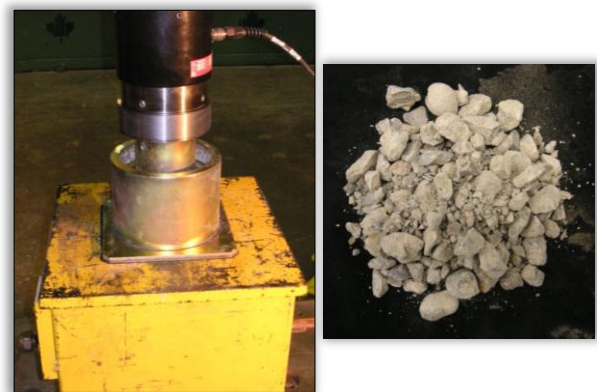
Testing crushing strength of RCA
