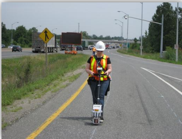
Measuring the longitudinal profile for MTO with the CPATT Surpro
