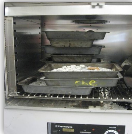
Innovative materials being prepared for testing, such as Recycled Concrete Aggregate
