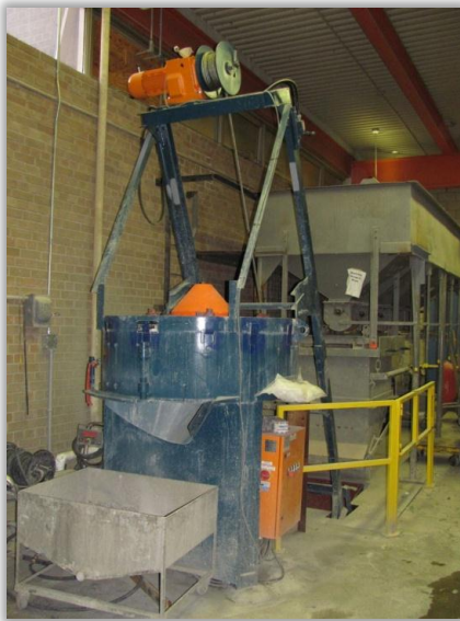
New Concrete Pan Mixer (8 cubic ft) (aggregate bins and hopper system in background)
