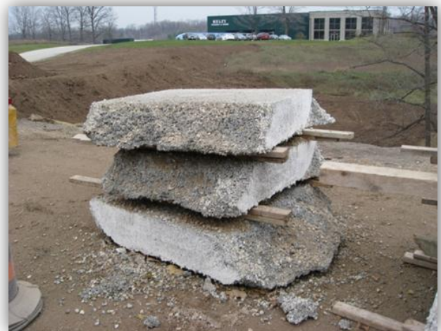
Pervious concrete slabs extracted during construction for laboratory testing
