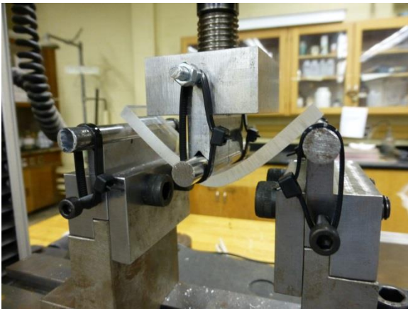
Three-point bending of a polycarbonate sample
