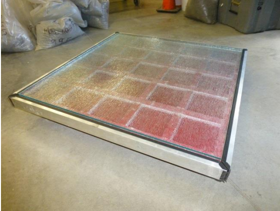
Solar road panel prototype for structural testing
