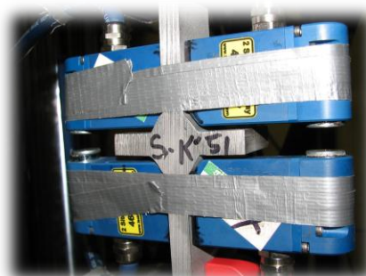
ACPD Probes for measuring fatigue crack growth at four critical locations for fatigue on cruciform weld specimen
