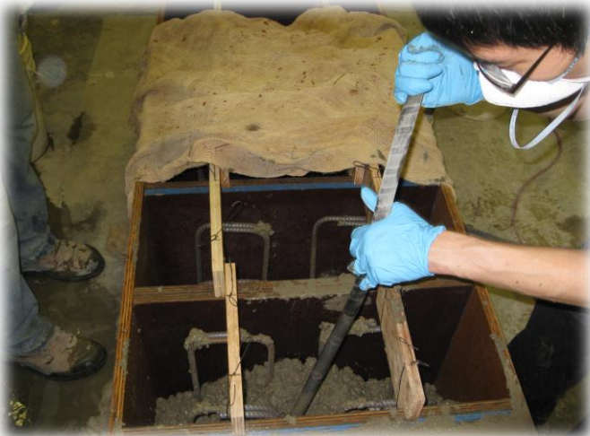
Consolidating beam end specimens for concrete with Recycled Concrete Aggregate (RCA)
