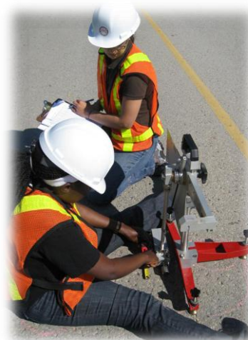
Friction Testing Using British Pendulum
