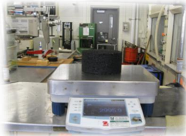
Bulk relative density test on Recycled Asphalt Shingles (RAS)
