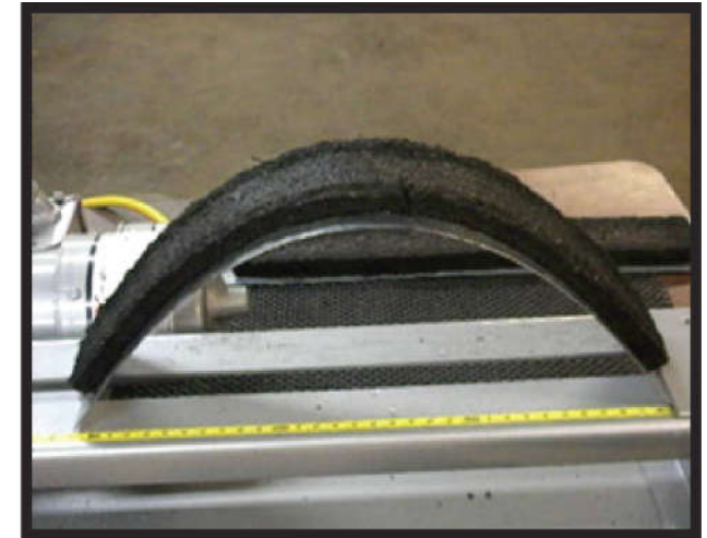
REINFORCED MIX 0.2% DOSAGE OF 1/4" SURFACE-EXT FIBER
