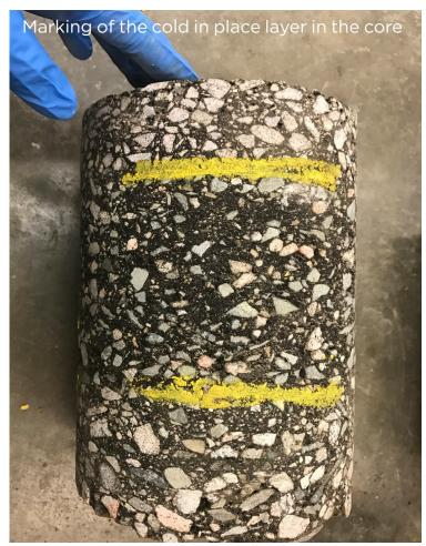
Dr. Torres-Matchi is currently working on different projects related to pavement sustainability in CPATT. One of those projects is comparing the performance of cold-in-place recycling with emulsion, versus expanded asphalt. As part of this project, pavement cores from different regions of Ontario are being evaluated at the CPATT lab.
